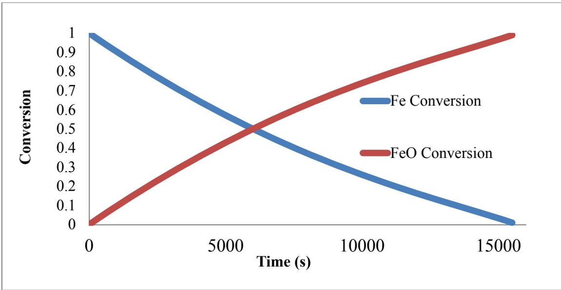
**Figure 4.6 : Fe and FeO conversion over time for 200mA/cm<sup>2</sup>**
