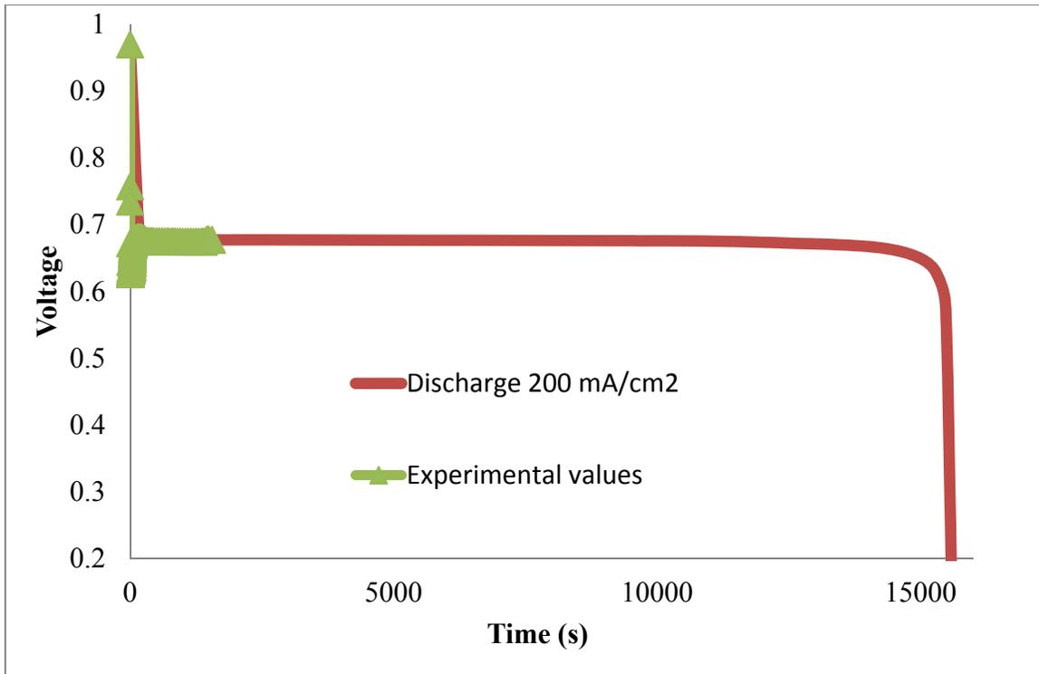
**Figure 4.1 : Discharge profile for 200mA/cm<sup>2</sup>**
