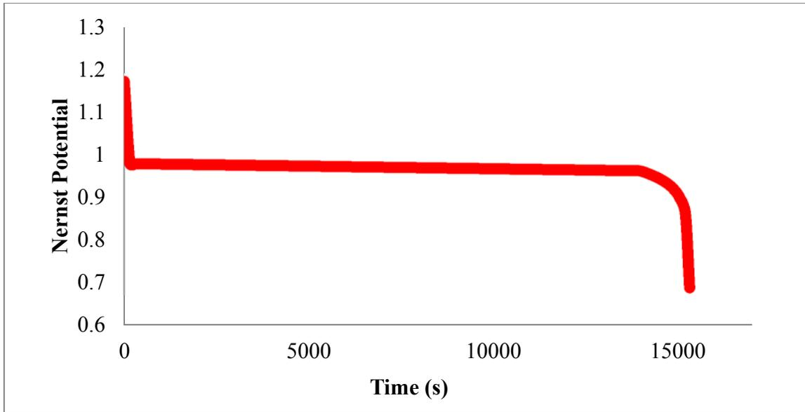
**Figure 4.2 : Nernst potential profile under 200mA/cm<sup>2</sup>**
