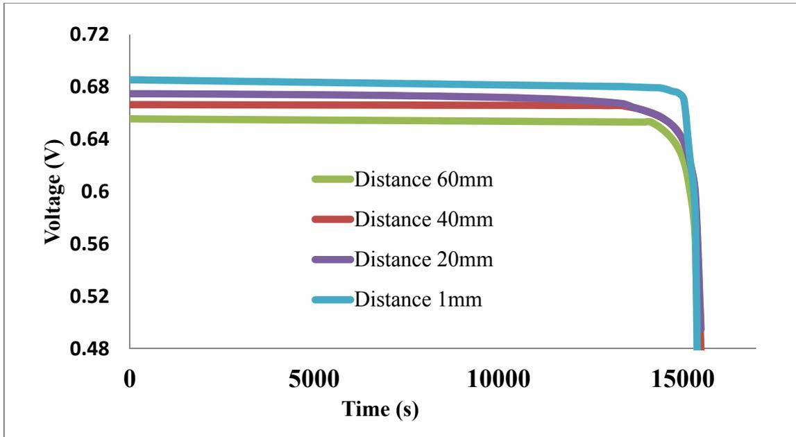
**Figure 4.11 : Discharge profiles for different free space variation.**
