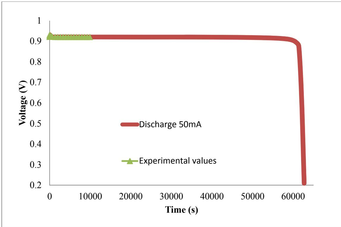
**Figure 4.4 : Discharge profile for 50mA/cm<sup>2</sup>**
