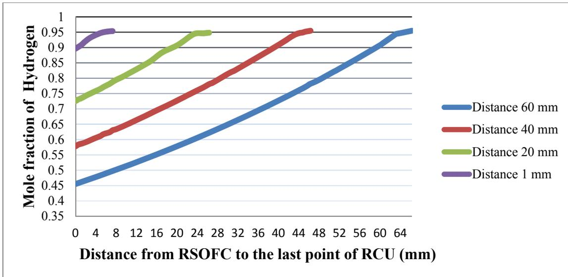
**Figure 4.10 : Hydrogen profile for different RSOFC-RCU distances**
