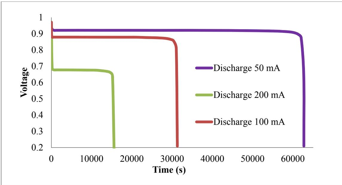
**Figure 4.8 : Discharge profile for different applied current densities**
