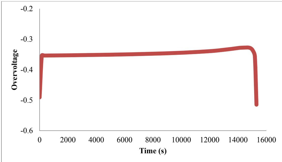
**Figure 4.3 : Overvoltage profile of the battery for 200mA/cm<sup>2</sup>**
