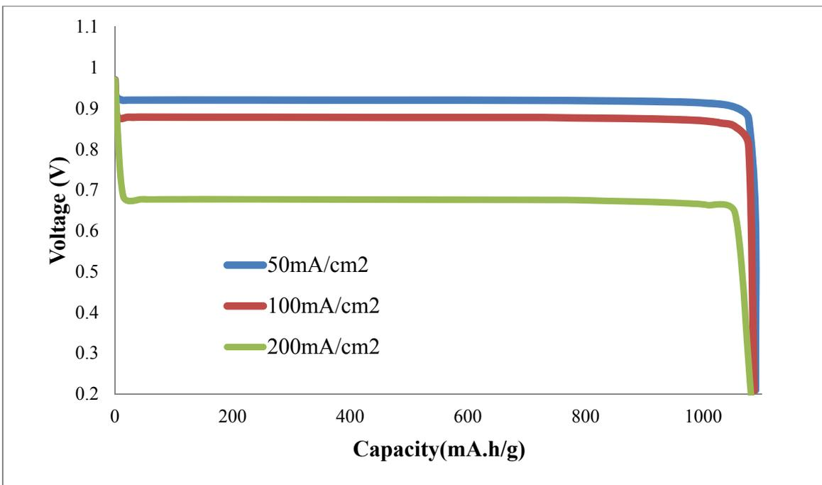
**Figure 4.9 : Capacity profile for different applied current densities**
