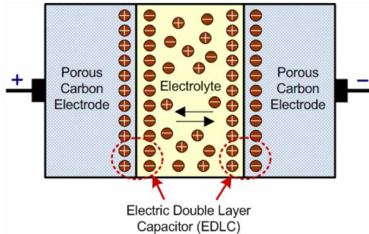
**Figure 1.2 : Schematic view of a Double Layer Capacitor**
