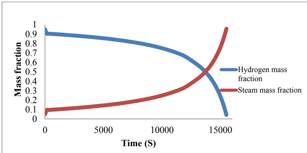
**Figure 4.5 : hydrogen and steam mass fraction over time**
