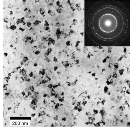
FIG. 1. Plan-view TEM image of an as-deposited  $\text{Fe}_{67}\text{Ga}_{33}$  thin film showing nanocrystalline morphology with an average grain size of 25 nm. The inset is a selected area diffraction pattern.
