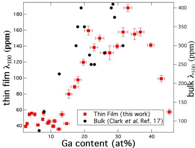
FIG. 2. (Color online)  $\frac{3}{2}\lambda_{100}$  measured from Fe–Ga thin-film composition spread plotted against values from previous bulk studies (Ref. 17) as a function of Ga content. The compositional trend and values agree well with bulk values. A third minor maximum is observed at a Ga concentration of 4.5 at. %. The error bars represent the standard deviation of the magnetostriction estimated from the experimental noise after smoothing and were taken at each measurement point.
