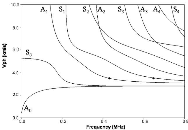
FIG. 8. Dispersion curves of 0.5 in. (12.7 mm) thick aluminum plate ( $c_P=6.2$  km/s,  $c_S=3$  km/s, and  $\rho=2.7$  gm/cc). Two black circles are the experimental data points corresponding to the two peaks at 430 kHz and 645 kHz in the  $V(f)$  curve of Fig. 5, corresponding phase velocity  $V_{ph}=3.526$  km/s for  $25^\circ$  angle of incidence is obtained from Snell's law [Eq. (2)]. Antisymmetric and symmetric modes of order  $m$  are denoted by  $A_m$  and  $S_m$ , respectively.
