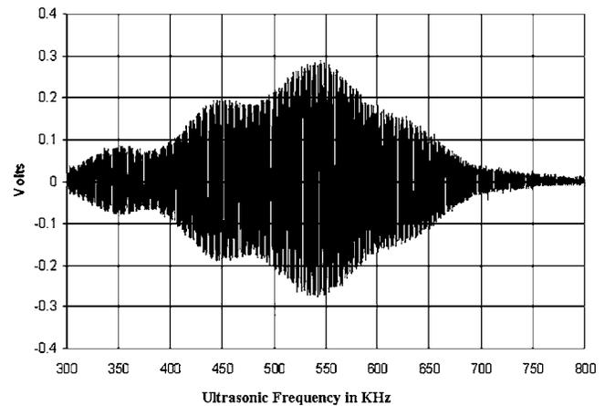
FIG. 4. Received signal voltage amplitude versus signal frequency curve, or  $V(f)$  curve, for a smooth plate specimen when the receiver is placed in the direct reflection zone marked by dashed lines in Fig. 3. Note the similarities between Figs. 1(b) and 4. [For this figure,  $\theta=25^\circ$ ,  $h=3$  in. (76.2 mm),  $d=2.8$  in. (71.1 mm), and the signal attenuation is 37 dB. A similar plot is obtained for  $h=2.5$  in. (63.5 mm) and  $d=2.3$  in. (58.4 mm)].
