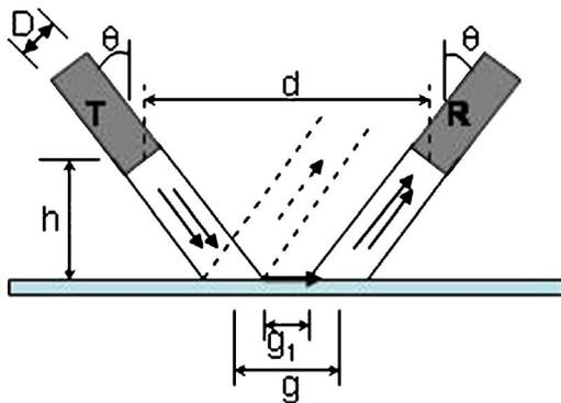
FIG. 3. Schematic of the transmitter ( $T$ ), receiver ( $R$ ) and the plate specimen arrangement. The direct reflected beam is shown by dashed lines. The receiver is placed beyond the direct reflection zone to detect the leaky guided waves.
