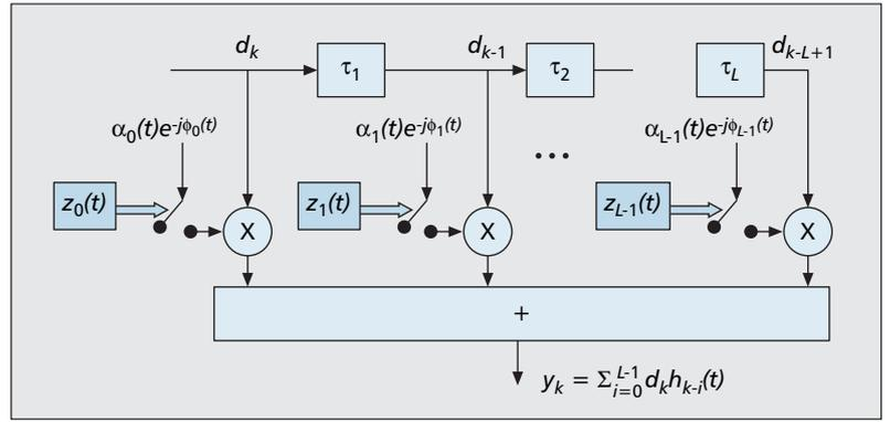
■ **Figure 2.** Tapped delay line model for a wireless channel, showing explicit multipath persistence (on/off) processes  $z_k(t)$ . Notation  $h_k(t) = \alpha_k(t) \exp[-j\phi_k(t)] z_k(t)$ ;  $k$ th switch is closed for  $z_k = 1$ , open for  $z_k = 0$ .
