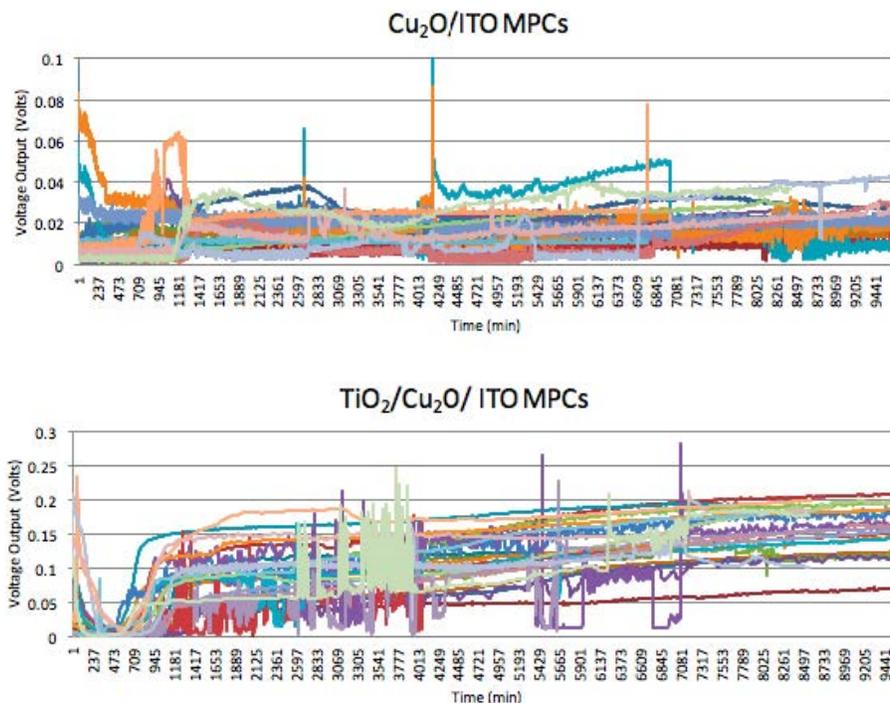
Figure 3: Graph of Fuel Cells' volts per minute. Graph of all fuel cell's volts per minute over approximately seven days. A visual trend shows that TiO<sub>2</sub>/Cu<sub>2</sub>O/ITO MPCs have higher voltage outputs compared to those of Cu<sub>2</sub>O/ITO MPCs. Also, the bacteria do not seem to completely stabilize across all fuel cells till after 5,000 elapsed minutes.
