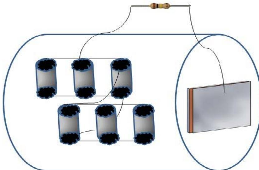
Figure 1. MPC Single Cell Prototype. Six anodic graphite electrodes were connected in a parallel circuit and were connected externally, through a 100 ohm resistor, to the TiO<sub>2</sub>/Cu<sub>2</sub>O/ITO photocathode. The anodic electrodes were placed in 1 liter of TSB media and the prototype was inoculated with a *Shewanella oneidensis* MR-1.
