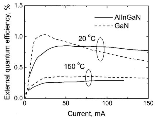
FIG. 4.  $\eta$ - $I$  characteristics of AlInGaN/InGaN and GaN/InGaN MQW LEDs.
