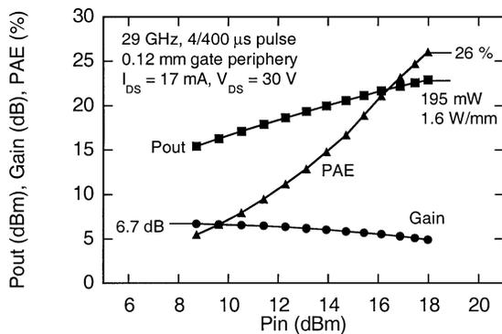
Fig. 5. Power performance of a 120- $\mu\text{m}$  gate-periphery AlGaN/GaN HEMT at 29 GHz. The pulsed on-wafer power measurements were performed using 4- $\mu\text{s}$  pulses and a 400- $\mu\text{s}$  duty cycle.
