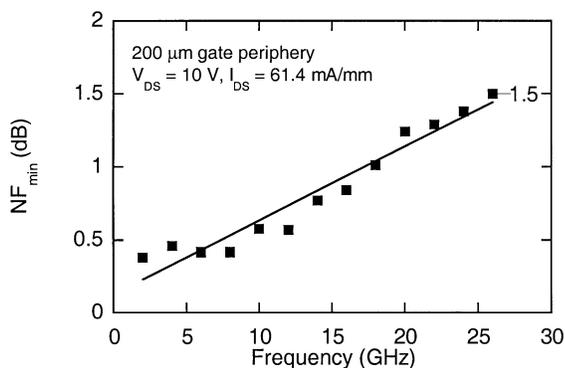
Fig. 6. Minimum noise figure versus frequency for the typical 0.2- $\mu\text{m}$  AlGaN/GaN HEMT with a gate periphery of 200  $\mu\text{m}$ . The solid line represents a linear fit to experimental  $\text{NF}_{\text{min}}$  data.
