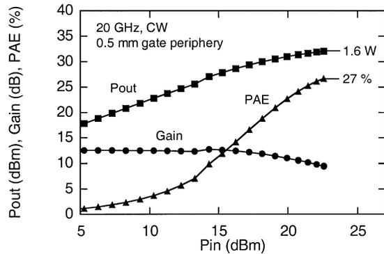
Fig. 4. Power performance of a 500- $\mu\text{m}$  gate-periphery AlGaIn/GaN HEMT showing a total CW output power of 1.6 W at 20 GHz. The device was biased at  $V_{\text{ds}} = 25$  V and  $I_{\text{ds}} = 200$  mA.
