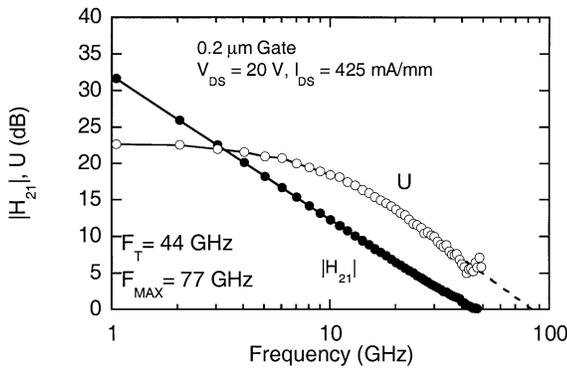
Fig. 2. Small-signal RF performance of a four-finger 200- $\mu\text{m}$  total gate-periphery AlGaIn/GaN HEMT. The unity current gain cutoff frequency ( $f_t$ ) and maximum oscillation frequency ( $f_{\text{max}}$ ) were determined to be 44 and  $\sim 80$  GHz, respectively.
