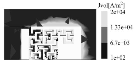
Fig. 6. Current distribution of antenna A at 2.45 GHz.
