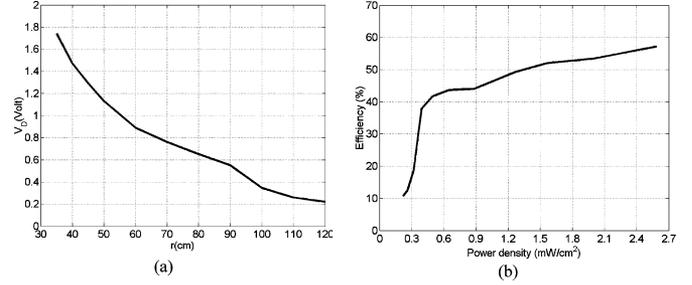
Fig. 9. Measured output voltage  $V_D$  and conversion efficiency of the CP rectenna at 5.5 GHz. (a) Distance versus output voltage  $V_D$ . (b) Power density versus conversion efficiency;  $R_L = 300 \Omega$ ,  $C = 68 \text{ pF}$ .
