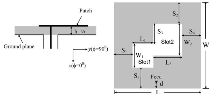
Fig. 1. Antenna geometrical configuration; cross section and top view. Antenna parameters:  $L = 14.8$  mm,  $W = 14.8$  mm,  $L_1 = 4.1$  mm,  $L_2 = 5.2$  mm,  $W_1 = 5.45$  mm,  $W_2 = 5.8$  mm,  $S_1 = 2.75$  mm,  $S_2 = 3.25$  mm,  $S_3 = 2.85$  mm,  $S_4 = 2.75$  mm,  $S_5 = 3.25$  mm,  $d = 2.83$  mm,  $h = 3.175$ ,  $\epsilon_r = 2.2$ .
