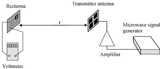
Fig. 8. Rectenna measurement setup.
