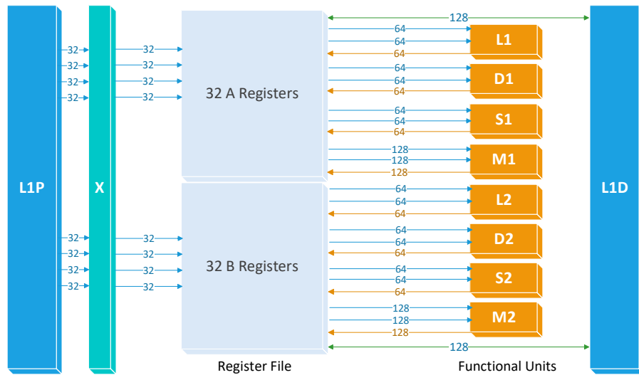
Figure 2.3 Simplified Texas Instruments C66x DSP Block Diagram [24]
