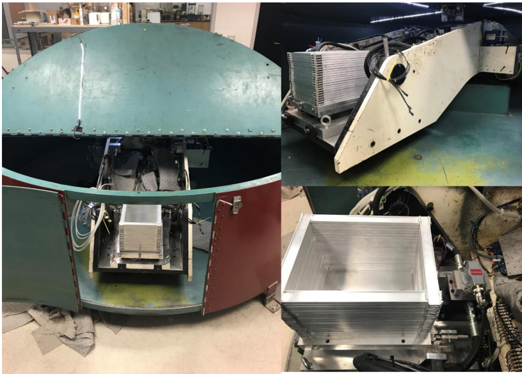
Figure 3.2 Pictures of centrifuge equipment, arm, and laminar box.
