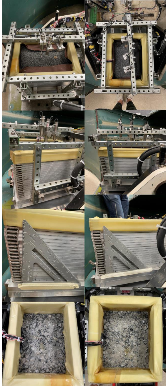
Figure 3.25 Post-test visual assessment of centrifuge models: (a) Cent1_L, and (b) Cent2_D.
