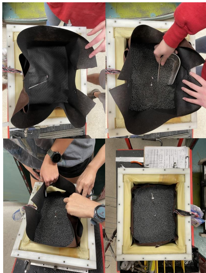
Figure 3.6 Geotextile and leadshot placement.
