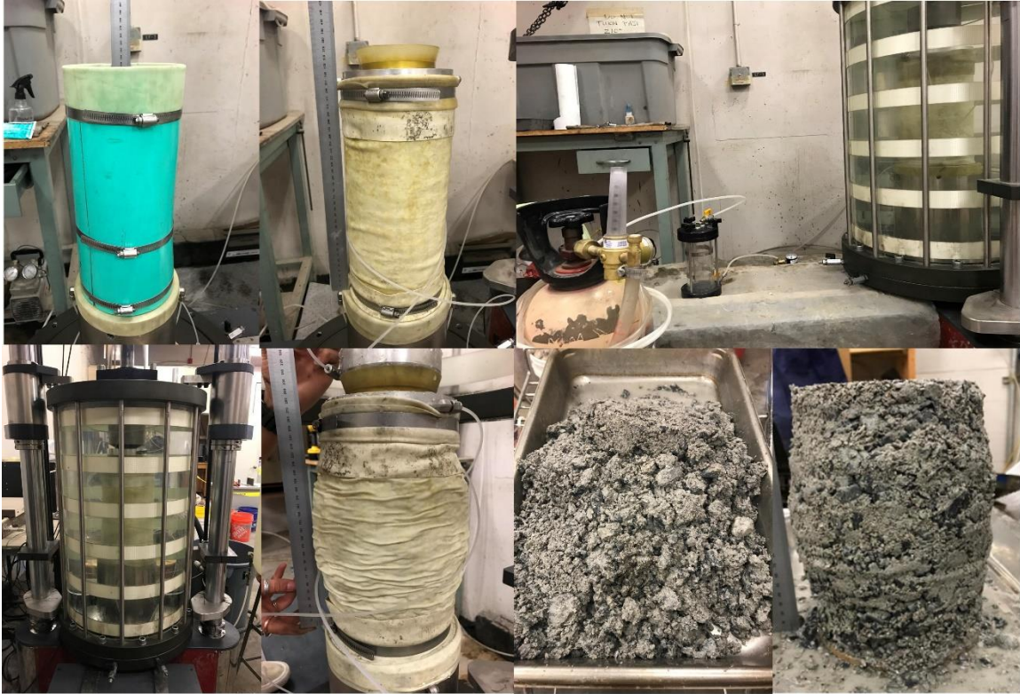
Figure 2.4 Pictures of sample preparation process and post-test observation for 6” sample diameter.
