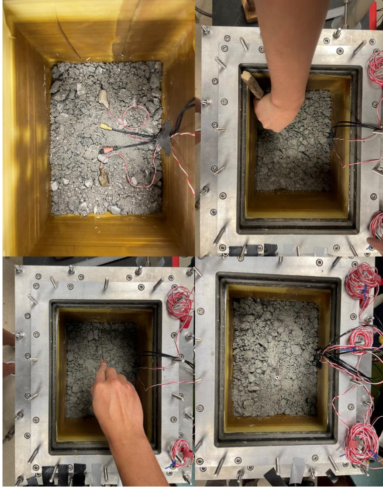
Figure 3.4 Model construction including sensor array within layer.
