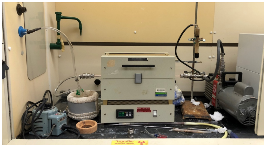
Figure 1.5. Reaction set up for synthesizing Ln 2 S 3
