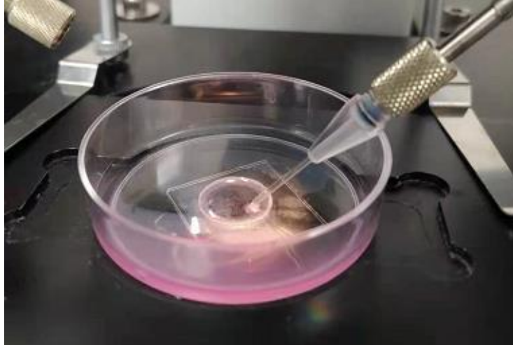
Figure 2.5: Injection system for Petri dishes experiments
