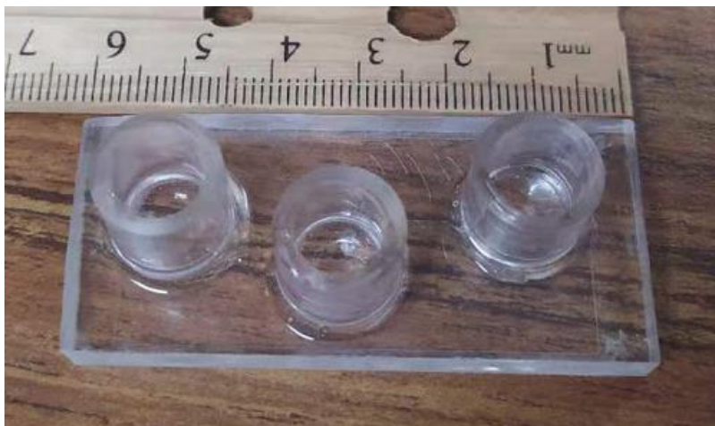
Figure 2.4: Completed microfluidics devices
