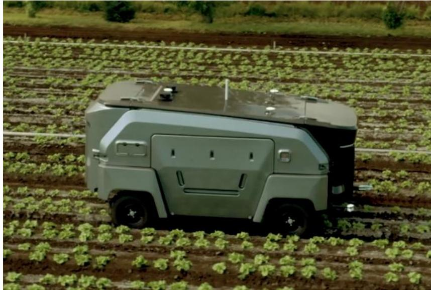
Figure 2.3: Nexus robot capable of picking weeds from the fields.
