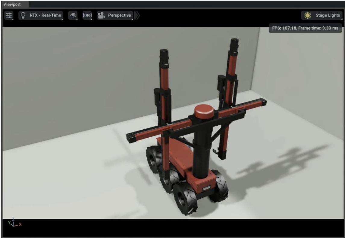
Figure 7.12: Digital-Twin of the StakeBot within Isaac Sim.
