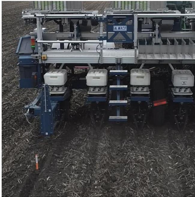
Figure 2.5 Stake Driver-Alley Marking System.
