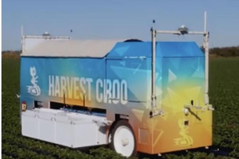
Figure 2.2: Harvest Croo’s robot capable of detecting and picking strawberries ready for harvest. (Harvest Croo Robotics)
