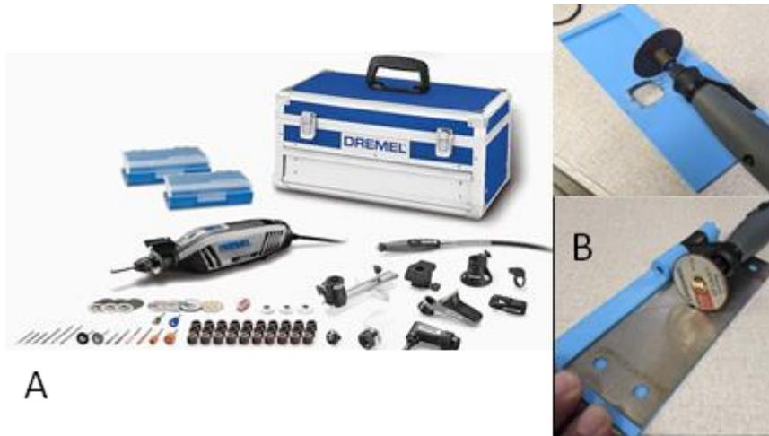
Figure 8.6 Tools used for crack starter cutting A) Dremel model 4300 76-piece variable speed corded multipurpose rotary tool with hard case purchased from Lowes.[28] (B, top and bottom) Sample cutting jig made of Blue PLA.
