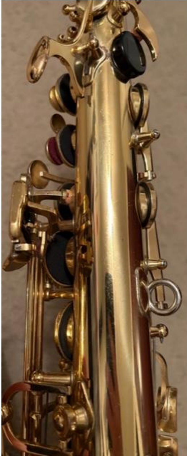
Figure 6.16: Foam pads applied to the left-hand stack of the test instrument.
