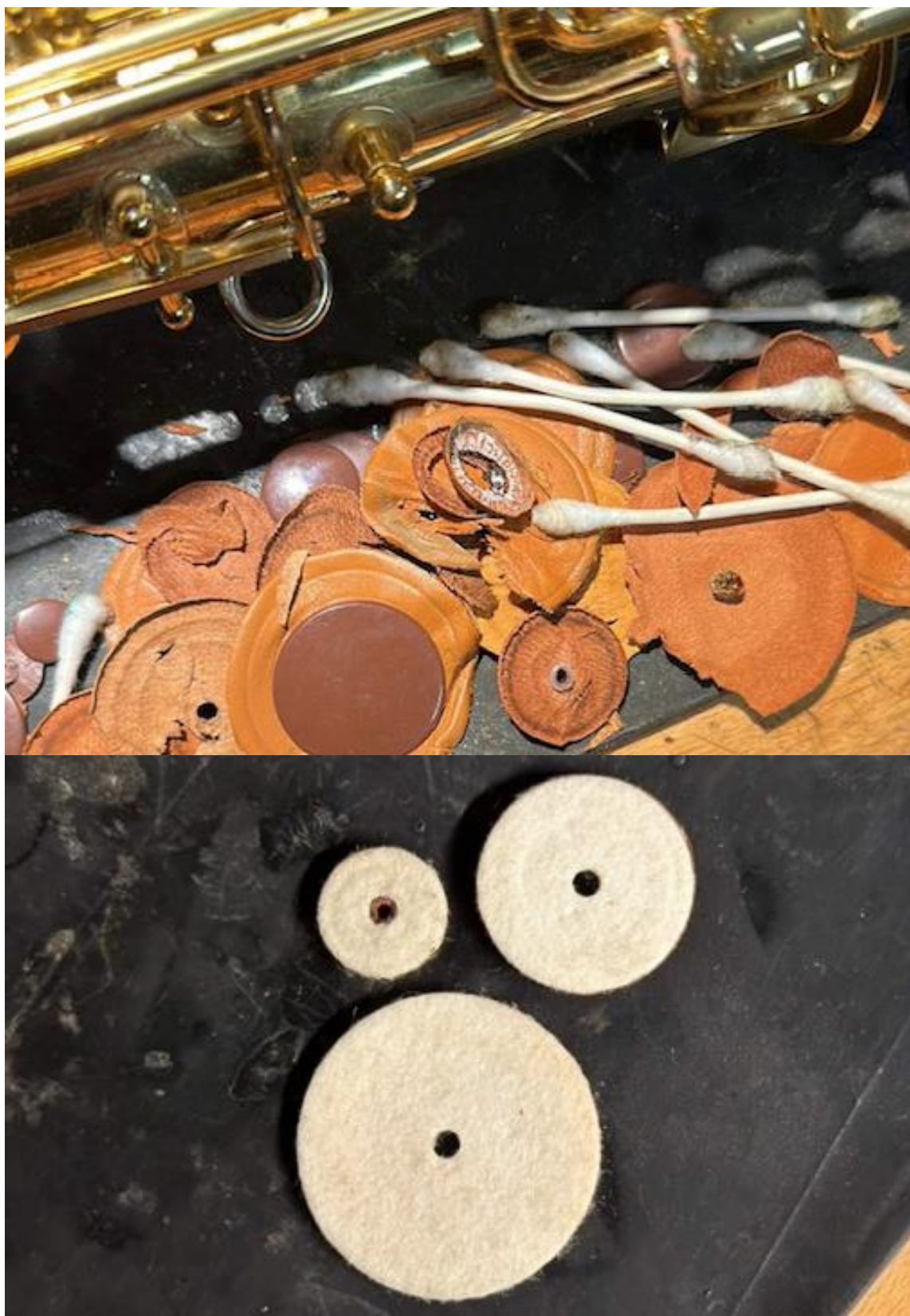
Figure 6.9: Removal of leather coverings and resonators of pads.
