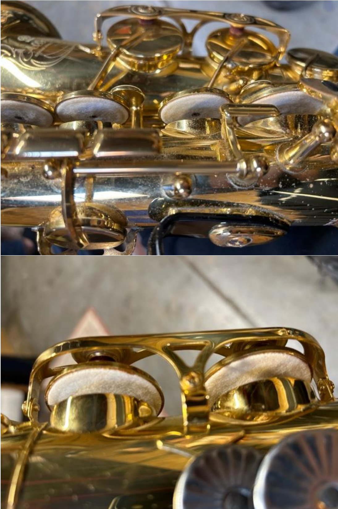
Figure 6.12: Removal of leather pad covering to expose felt layer.
