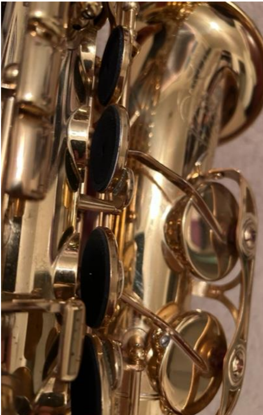
Figure 6.15: Foam pads applied to the right-hand stack of the test instrument.
