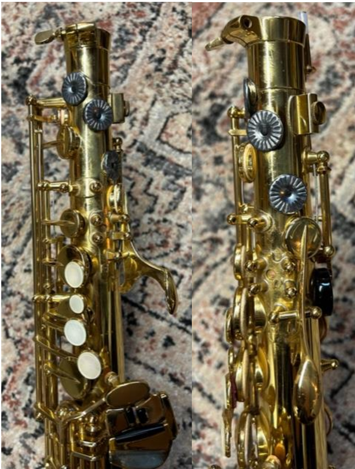
Figure 6.11: Removal and plugging of C2 and C4 keys (high D#/Eb and F).
