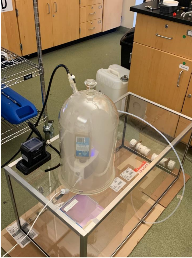
Figure 3.1 Nebulizer under bell jar hooked to vacuum pump and filter to collect aerosols for later analysis.
