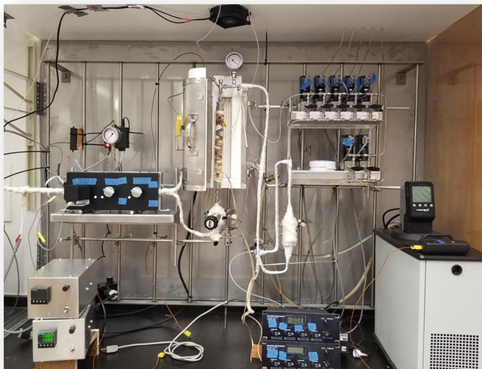
Figure 2.4. An image of a Flow system used for catalyst evaluation
