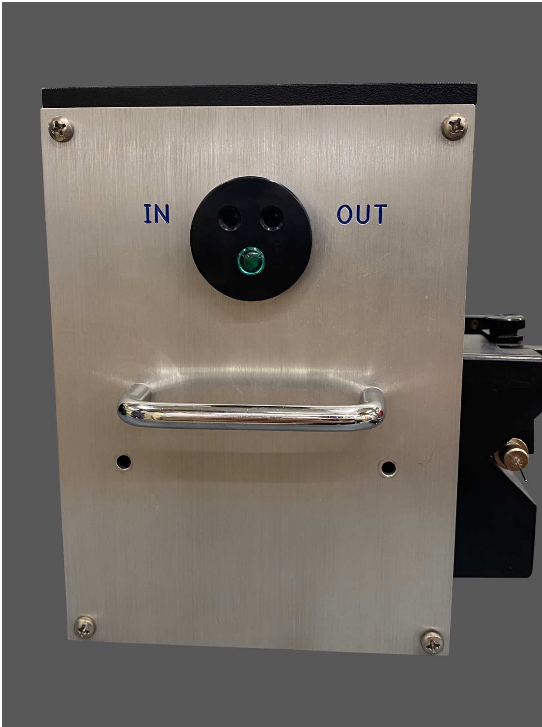
Figure 5.2 External View. The front of the Coagulation Companion has the openings “IN” for substrates entering the detection system and “OUT” for the waste.
