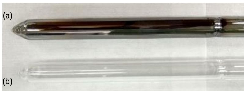
Figure 2.5 Carbon coated (a) and uncoated (b) quartz ampoule.
