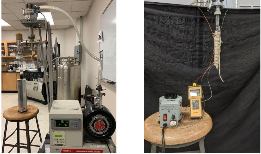
Figure 2.6 Quartz ampoule sealing system at our laboratory for growing CZTS crystals (left) and the growth ampoule being heat treated for sealing (right).
