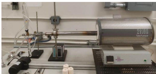
Figure 2.4 Tube furnace used for carbon coating in our lab.
