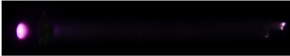
**Figure 2.2** Plasma discharge structure showing negative glow and weak positive column
