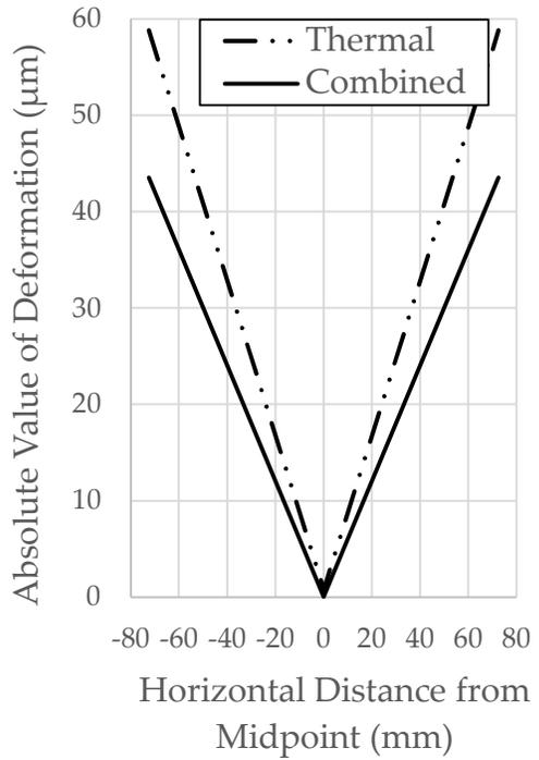
Figure 4.12: Transverse deformations (m) along (c) weld cross-section path for (a) thermal and (b) combined
