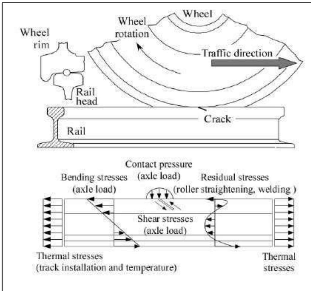
Figure 2.6: Stress diagram for typical rail [34]
