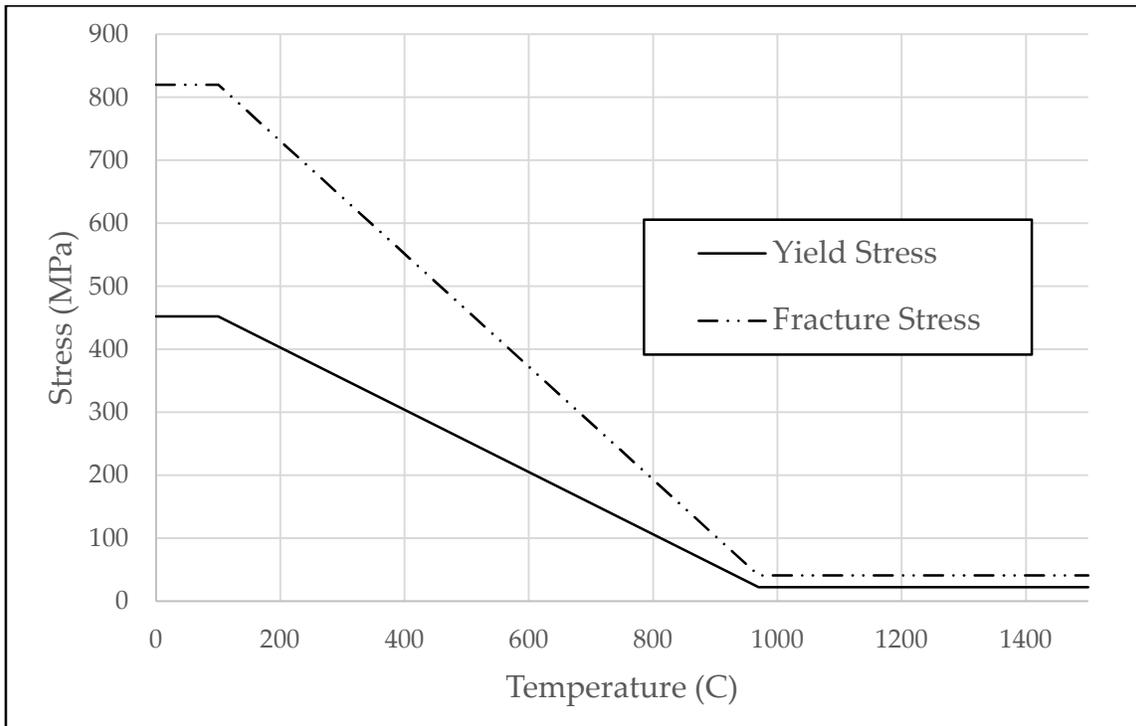
Figure 3.6: Simplified temperature-dependent yield and fracture stresses
