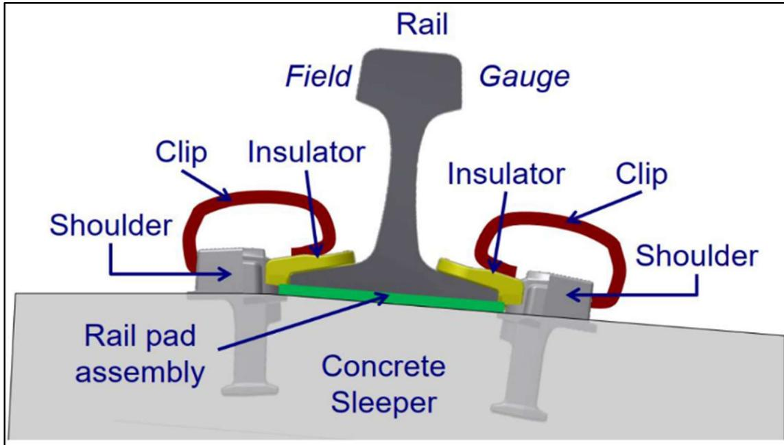
Figure 3.3: Cross-sectional view of clip style fastener system [6]
