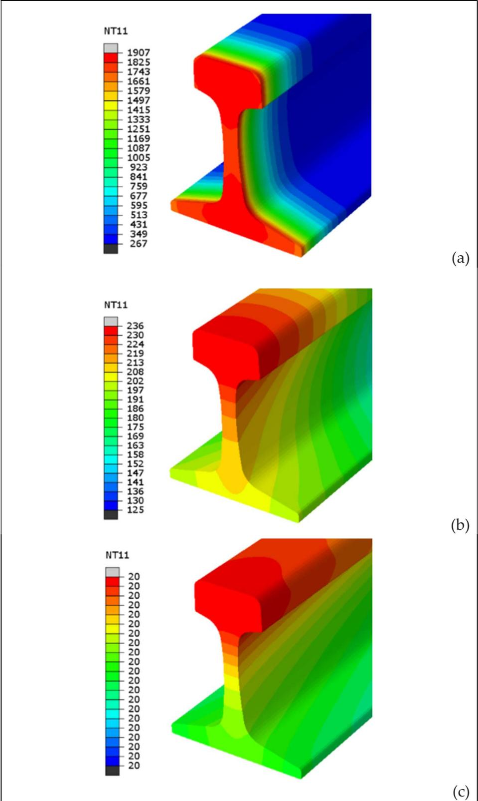
Figure 4.3: Weld fusion line temperature field evolution during welding ( $^{\circ}\text{C}$ ) at (a) 70 sec, (b) 1 000 sec, and (c) 10 000 sec
