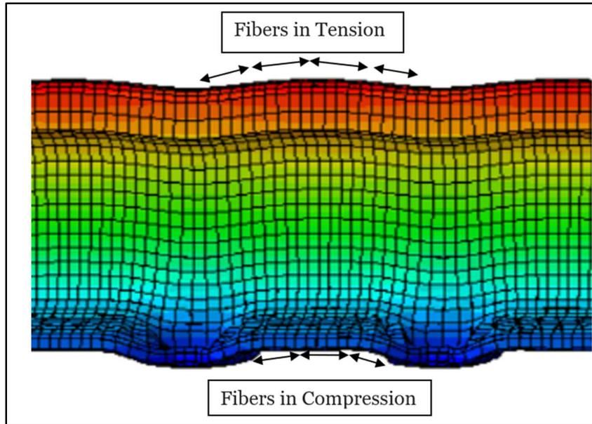
Figure 5.1: Beam bending of rail between sleepers
