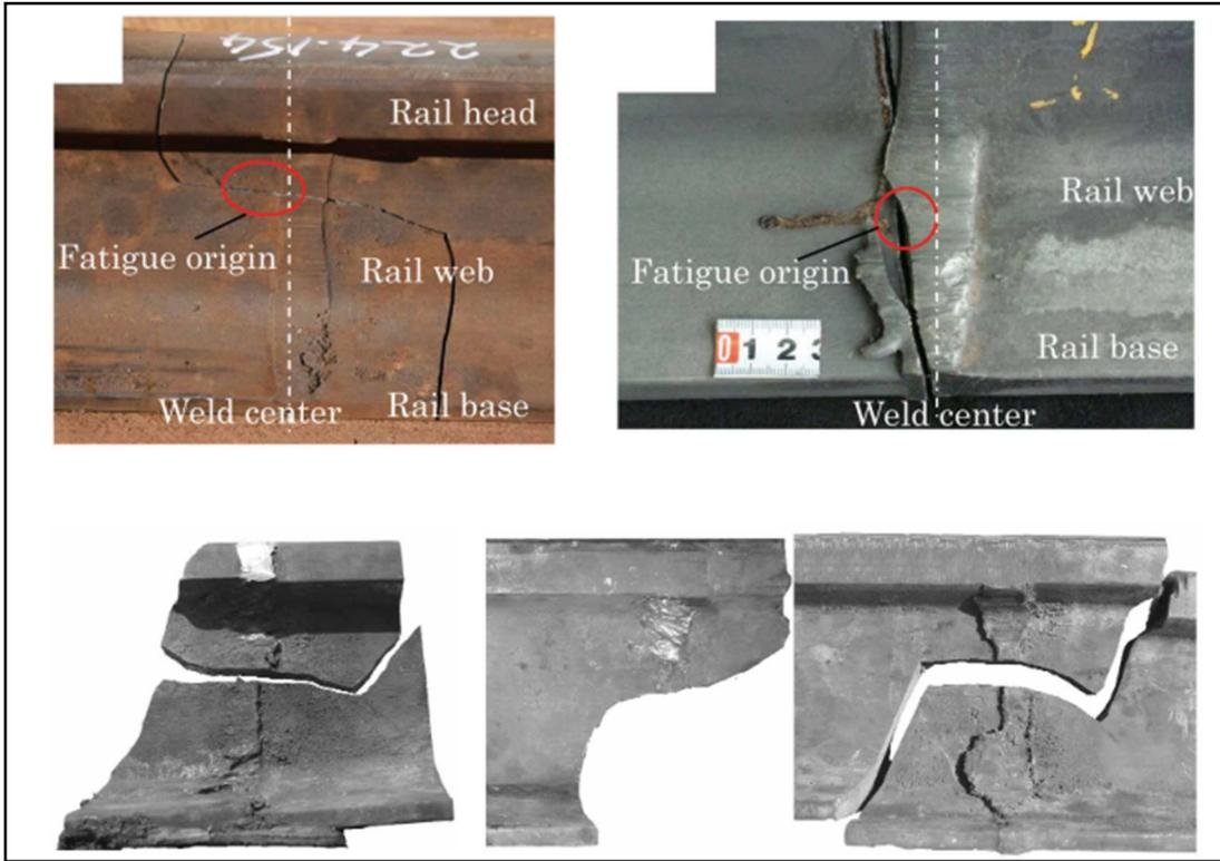
Figure 2.7: Fatigue cracking in flash-butt welds [33]
