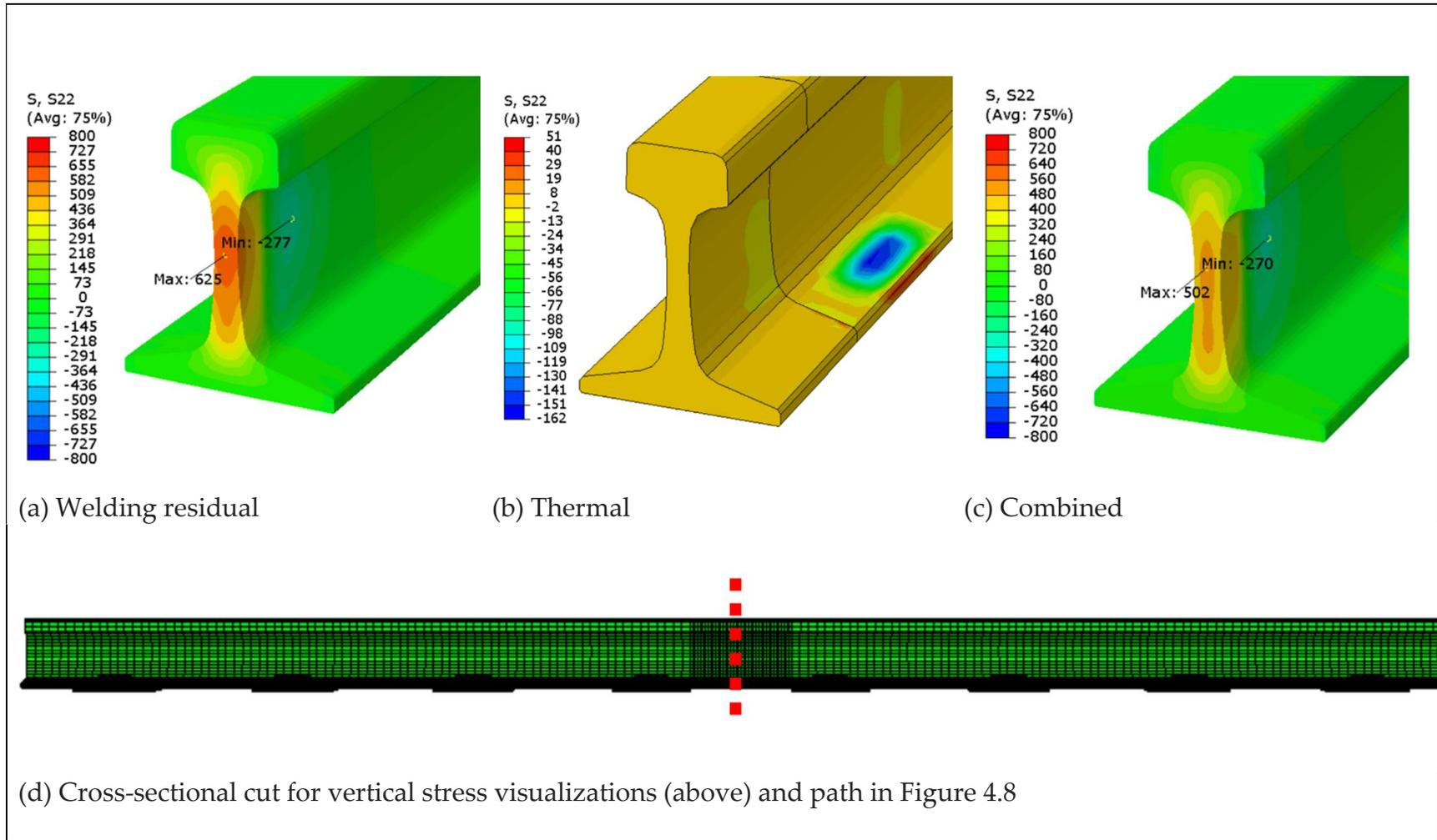
Figure 4.7: Vertical stress visualizations (MPa) at (d) weld cross-section for (a) welding residual, (b) thermal, and (c) combined
