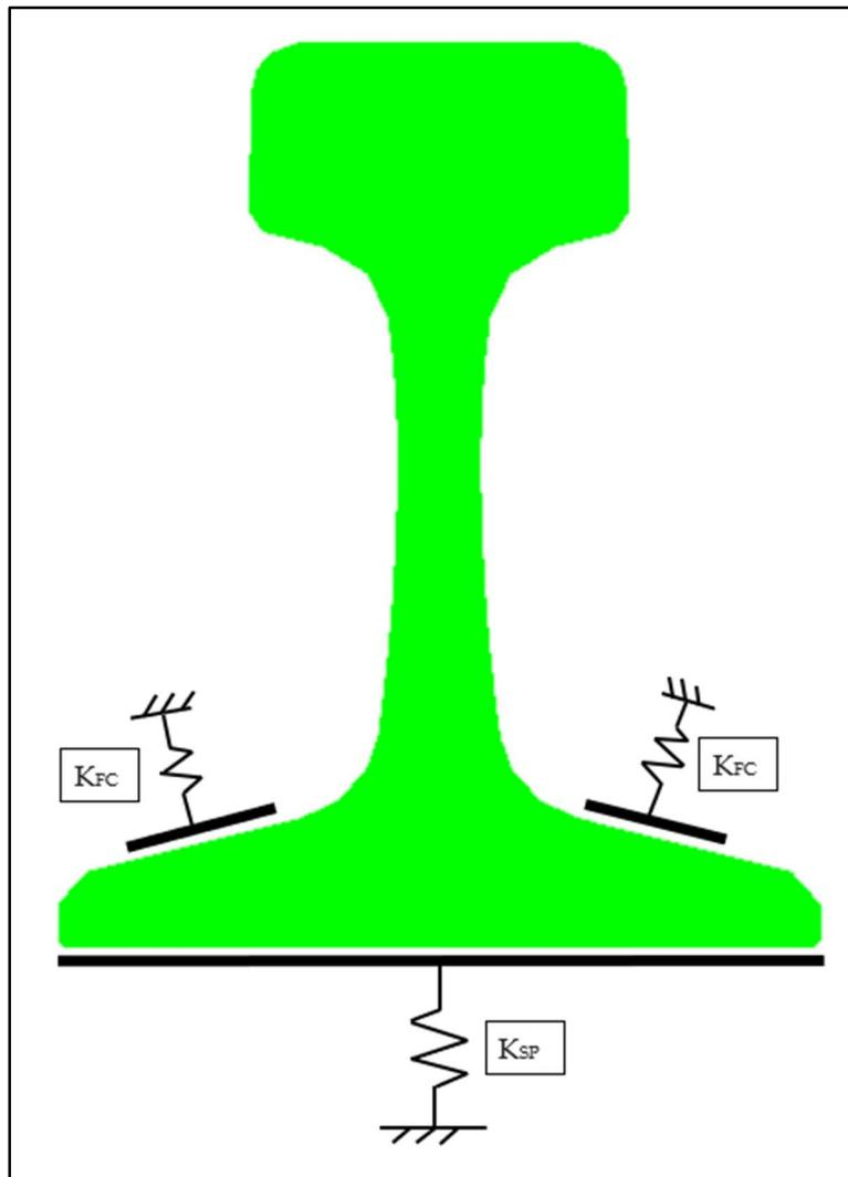
Figure 3.9: Simplified sleeper plate and fastener systems
