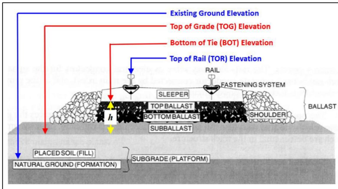
Figure 3.2: Cross-sectional view of typical rail foundation [6]
