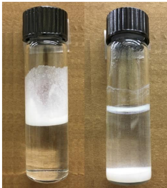
Figure 2.6 (left) Monolith polymers with 0 mol% NVP feed percentages having poor wettability floating on top of the aqueous solution after shaking (right) and monolith polymer with 30 mol% NVP feed percentages having good wettability and falling to the bottom of the aqueous solution.
