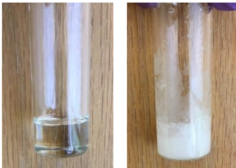
Figure 4.2 (left) DBU in methanol before bubbling CO 2 (right) [DBUH + ][HCO 3 - ] formed after bubbling in CO 2 for 10 minutes.
