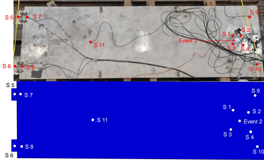
Figure 3.12 Finite element model representation for steel specimen
