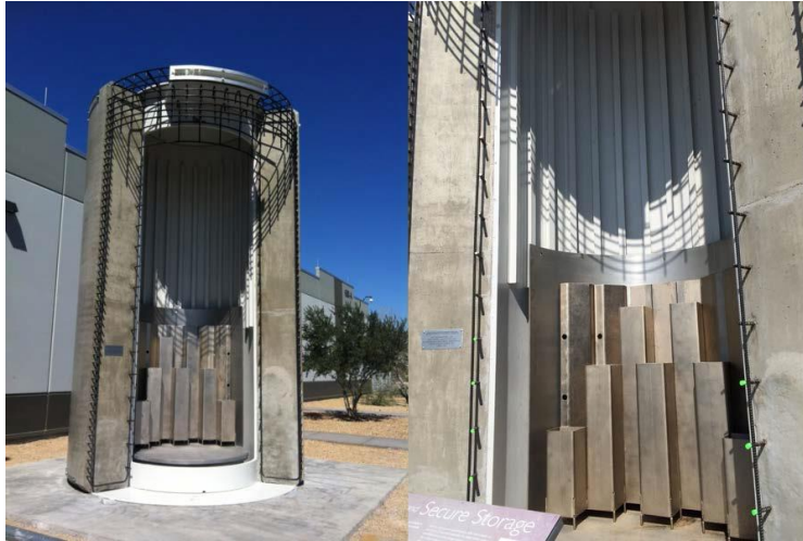
Figure 4.1 Cutaway mockup of simulated dry storage cask system
