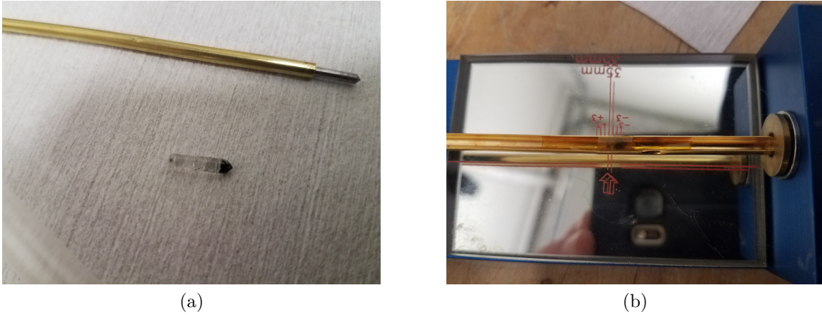
Figure 4.17 VSM Samples: a) VSM sample next to a diamond scribe and b) sample placed in the brass VSM sample holder.
