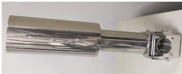
Figure 3.3 Vacuum shroud of the cryostat.
