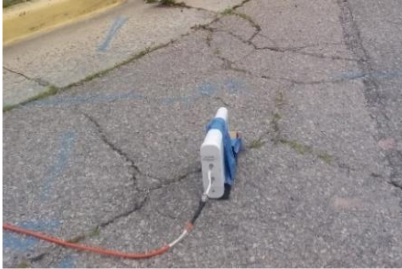
Figure 3.9. Transmitting antenna (log-periodic) on the ground aimed at the receiver in the car 100 m away.
