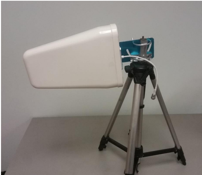
Figure 3.7. Log-periodic antenna mounted on tripod.
