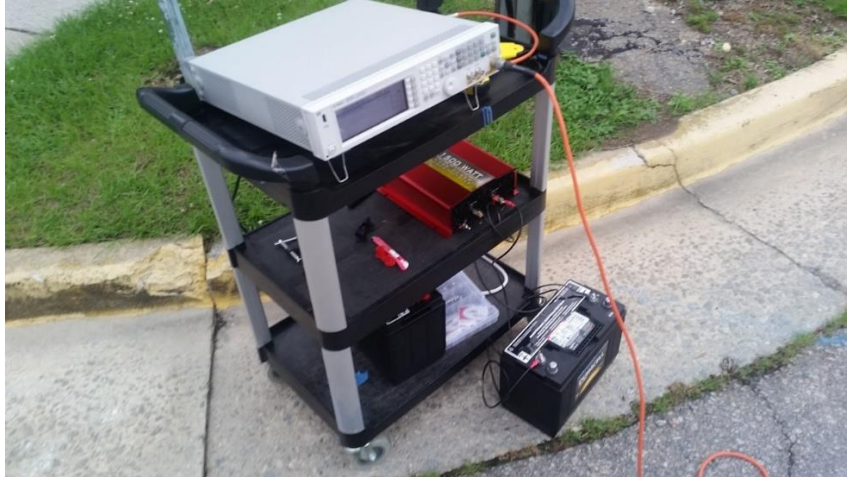
Figure 3.6. Signal generator, power inverter and car battery.
