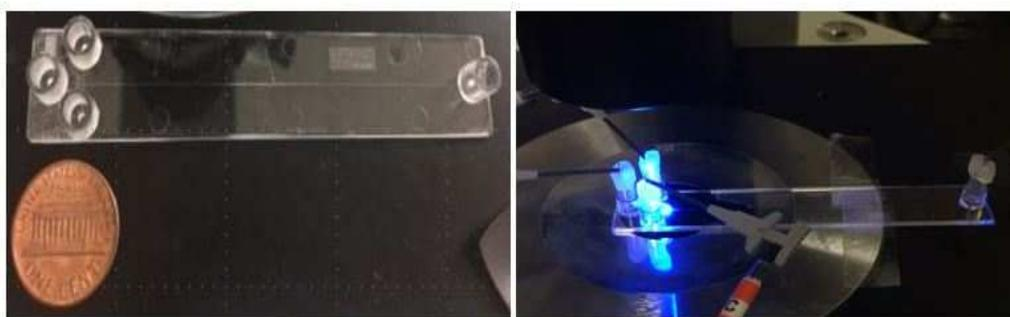
Figure 1. 1 A microfluidic chip performing the electrophoresis.
