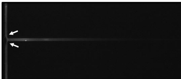
Figure 4. 1 Sample is leaking into separation channel after the sample injection is done under the separation voltage of 1000 V.
