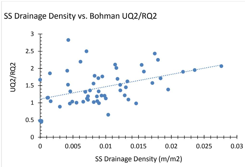
Figure 3.5 Ratios of Urban 2-year floods to rural 2-year floods as a function of corresponding SS drainage densities for the 58 subcatchments in RBW.  $UQ_2$  and  $RQ_2$  were computed using Equations 2 and 3 (Bohman 1992)
