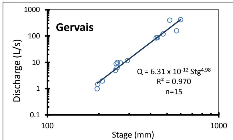
Figure 2.2 Stage-discharge rating curve for Gervais (Hung, 2018).
