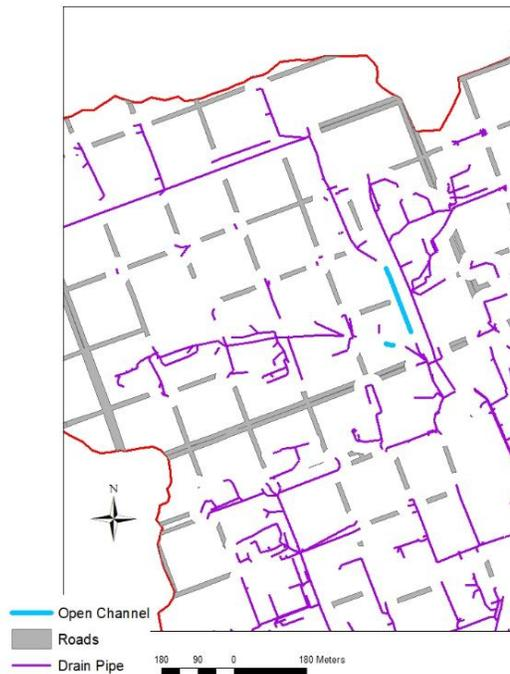
Figure 2.1 Detailed map of road-side gutters and ditches (bold lines), open channels, and storm sewers.
