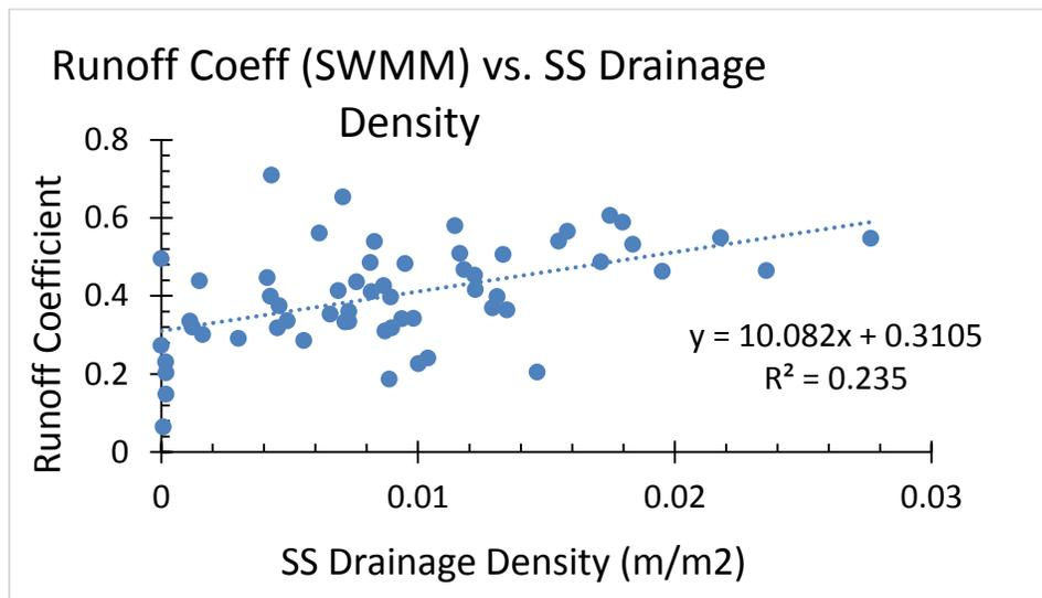
Figure 3.8 ROC values computed by SWMM model compared to SS Density.
