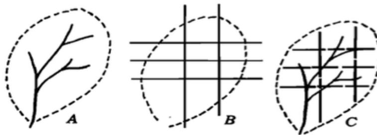
Figure 1.1: Drainage Configurations. Natural (A) and artificial (B) networks may be combined in an urban (C) watershed.
