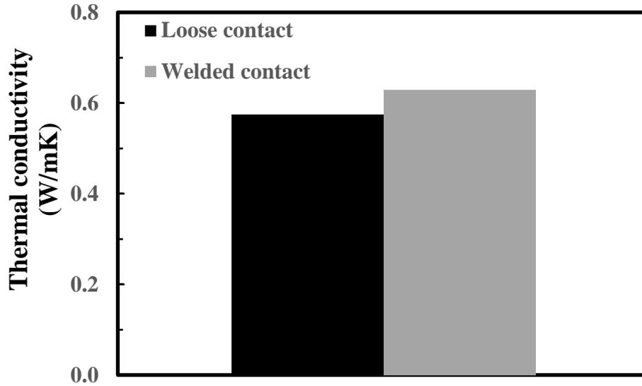
Figure 3.1: Effect of the nature of contacts between the foils on the  $k_{eff}$  perpendicular to the structure bed layers with the bed containing loose foils with zero gap (Run 1) and imbedded foils (Run 2) having 50  $\mu\text{m}$  foils with air as gas medium.
