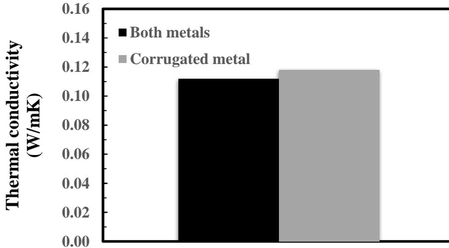
Figure 3.8: Effect of having pre-assembly adsorbent coating of 30  $\mu\text{m}$  in thickness on both the metal foils (i.e., run 10) and only on the corrugated metal foils (i.e., run 20) of 50  $\mu\text{m}$  in thickness with air as the medium.
