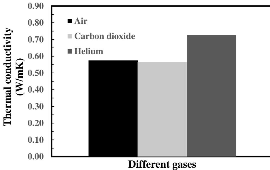
Figure 3.2: Effect of the different gas media (i.e., 1, 3, and 4) on the  $k_{eff}$  perpendicular to the structure bed layers with the bed containing loose metal foils in contact of 50  $\mu\text{m}$  thickness.
