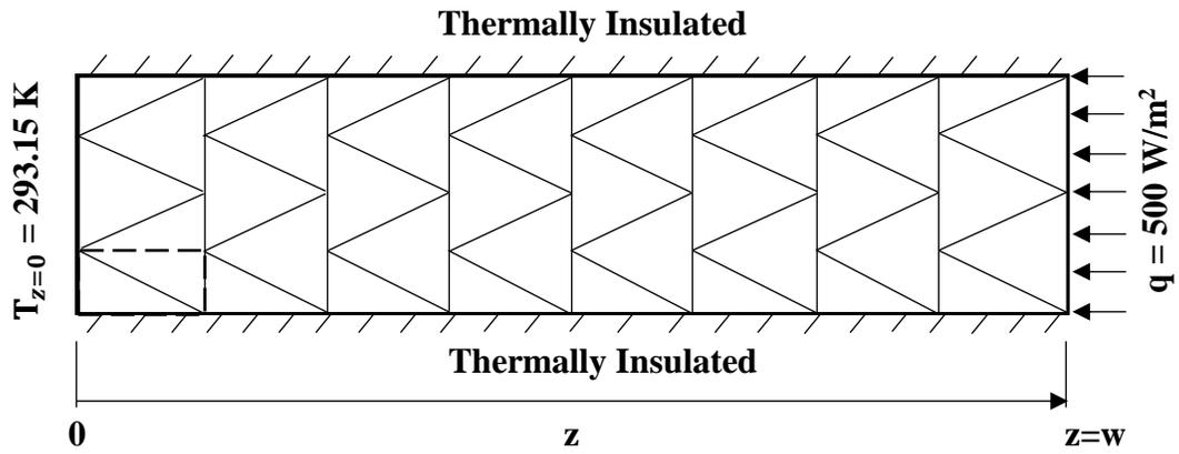
Figure 2.1: Control volume of the model using 8 layers of intercalated coated corrugated and 9 layers of smooth metal foils using a gas with the boundary conditions. The unit cell is highlighted at the bottom left corner of figure. Unit cells for each of the cases studied are magnified and represented in Figure 3.2.
