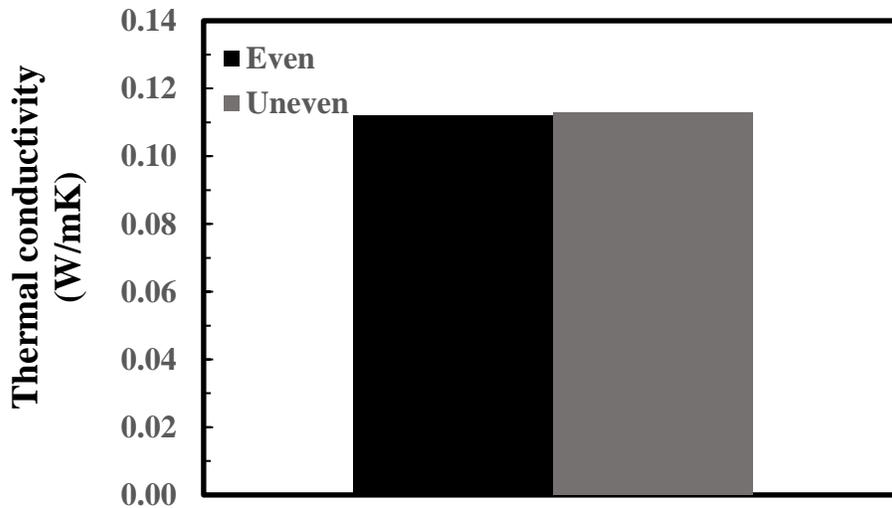
Figure 3.10: Effect of the alignment on the  $k_{eff}$  perpendicular to the structure bed layers with the bed containing metal foils of 50  $\mu\text{m}$  in thickness (i.e., runs 10, and 24) having 30  $\mu\text{m}$  coating with air as the medium.
