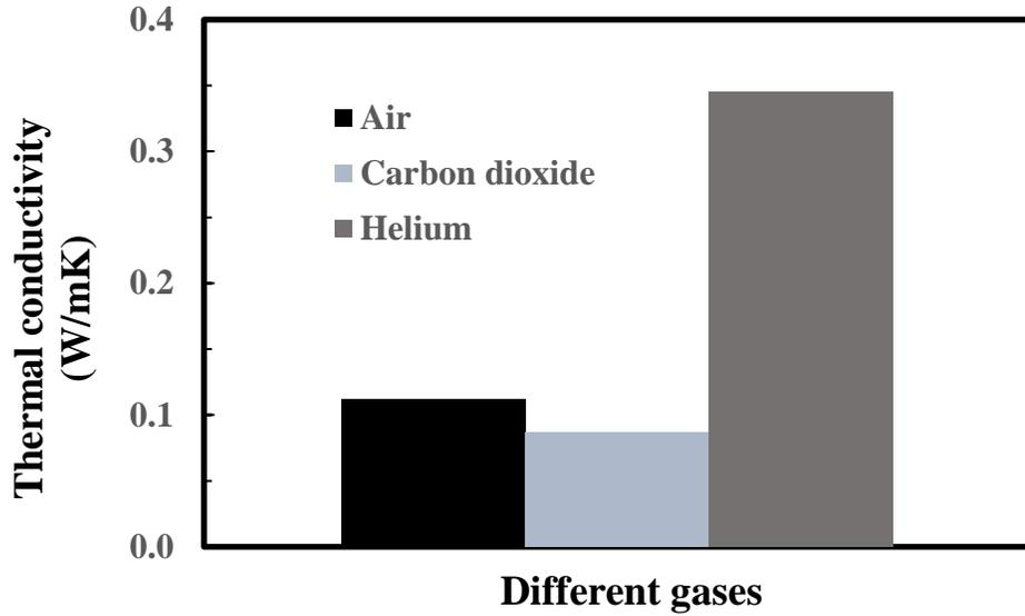
Figure 3.5: Effect of the different gas media (i.e., runs 10, 11 and 12) on the  $k_{eff}$  perpendicular to the structure bed layers with the bed containing metal foils of 50  $\mu\text{m}$  in thickness with 30  $\mu\text{m}$  coating thickness.
