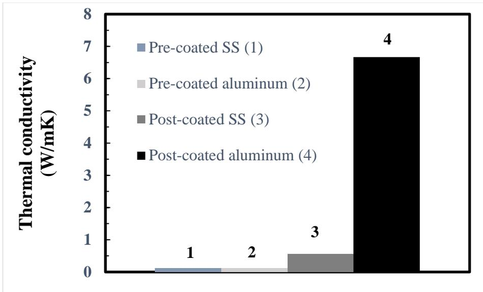
Figure 3.9: Effect of using different metals for the foils of structure bed layers on the  $k_{eff}$  with the bed containing 50  $\mu\text{m}$  in thickness foils with pre-assembly 30  $\mu\text{m}$  coating (i.e., runs 10, and 21) and post- assembly 30  $\mu\text{m}$  coating (i.e., runs 22, and 23) with air as the medium.
