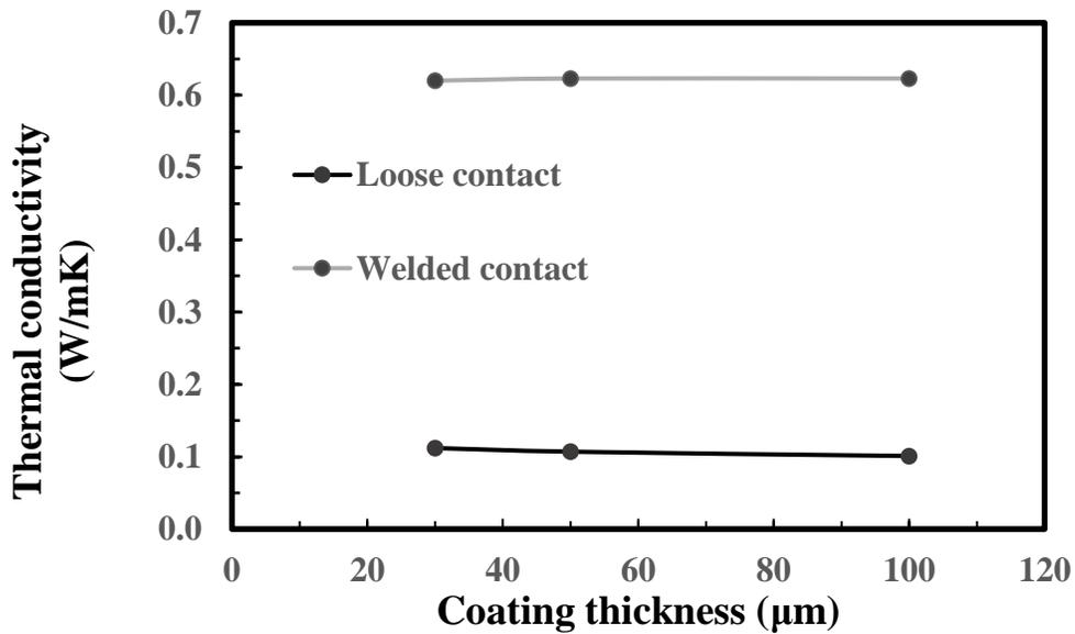
Figure 3.6: Effect of the thickness of adsorbent coating  $\delta_a$  of 30, 50 and 100  $\mu\text{m}$  on the  $k_{eff}$  perpendicular to the structure bed layers on both the metal foils of 50  $\mu\text{m}$  thickness having loose (i.e., runs 10, 13 and 14) and imbedded contacts (i.e., runs 15, 16 and 17) between them with air as the medium.
