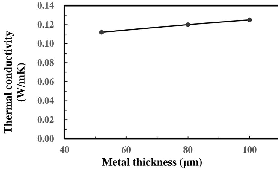
Figure 3.7: Effect of the metal thickness  $\delta_m$  on the  $k_{eff}$  perpendicular to the structure bed layers with the bed containing metal foils of 50, 80 and 100  $\mu\text{m}$  in thickness (i.e., runs 10, 18 and 19) with 30  $\mu\text{m}$  coating thickness with air as the medium.
