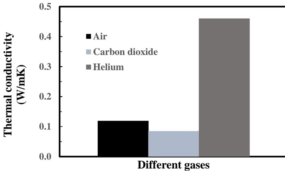
Figure 3.4: Effect of the different gas media on the  $k_{eff}$  perpendicular to the structure bed layers with the bed having 10  $\mu\text{m}$  gap (i.e., runs 5, 8 and 9) between the metal foils of 50  $\mu\text{m}$  thickness and no coating.
