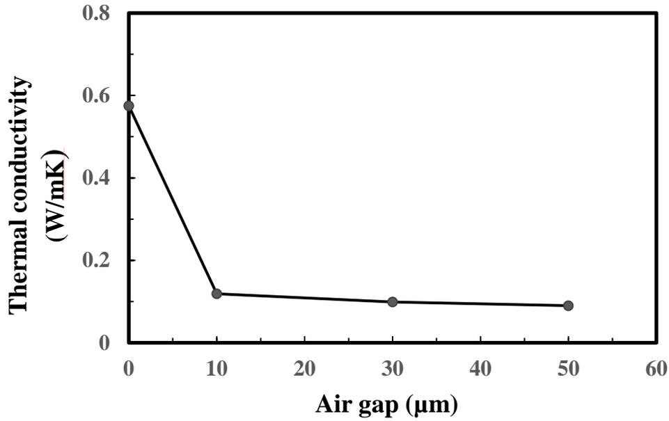
Figure 3.3: Effect of the air gaps  $\delta_g$  between the smooth and corrugated foils on the  $k_{eff}$  perpendicular to the structure bed layers with the bed containing gaps of 0, 10, 30, 50  $\mu\text{m}$  (i.e., runs 1, 5, 6 and 7) between the metal foils of 50  $\mu\text{m}$  thickness.
