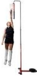
Figure 3.6. Vertec Jumping Apparatus
