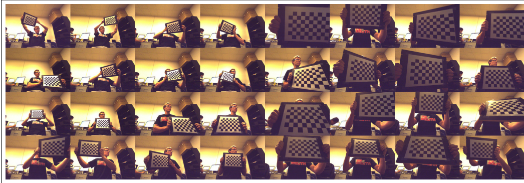
Figure 1.3: A collection of good viewing angles and distances for a calibration board
