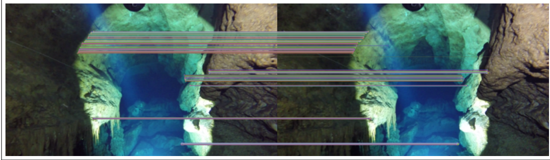
Figure 2.3: Select features matched at the boundary between left and right image of a stereo pair.
