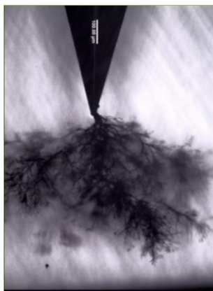
Figure 3.1. Optical microscopy image of tree formed as a result of avalanche breakdown in epoxy resin.
