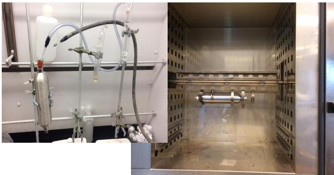
Figure 5.4. Experimental set-up for kilogram scale synthesis of PIP grafted NPs.
