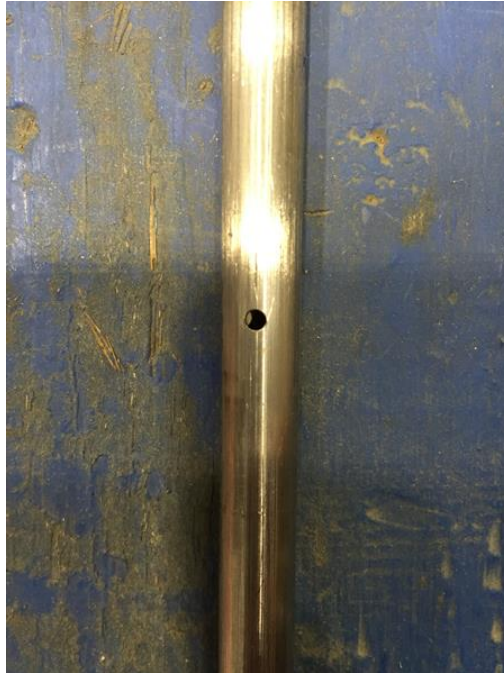
Figure 3.4 Defect on a mock failed fuel rod.
