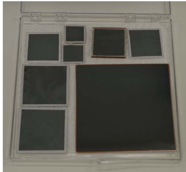
Figure 2.10. Enriched ^{10}\text{B} -doped a-Se (As, Cl) thin films deposited on Al/ \text{Al}_2\text{O}_3 substrates ( 4 \times 4 , 2 \times 2 , 1.5 \times 1.5 , and 1 \times 1 sq. inches) in a single deposition run grown in the modified evaporation system with larger mounting capabilities in the vacuum chamber.
