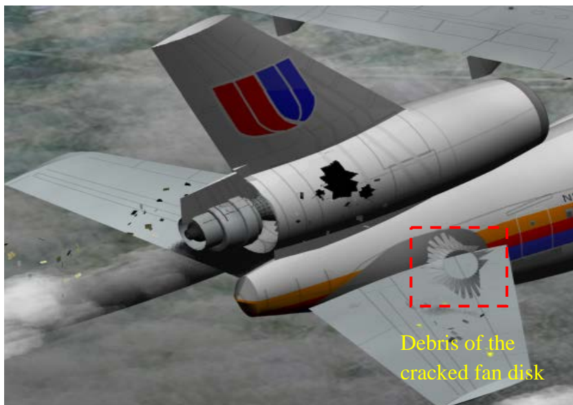
Figure 1.2: The debris of the failed fan disk came out of the engine nacelle [4]
