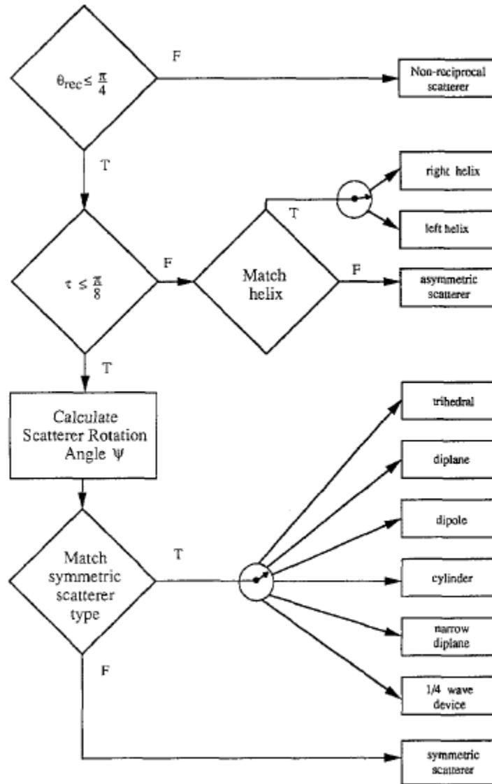
Figure 3.1 Scattering Matrix Classification Scheme from Cameron [1]
