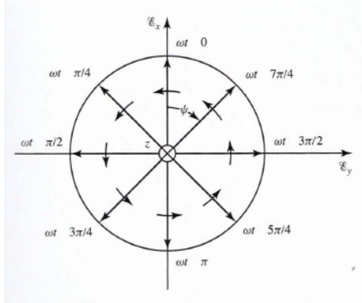
Figure 1.5 Left-Hand Circularly Polarized Wave from Balanis [9]
