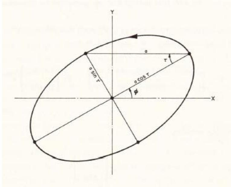
Figure 2.2 Left Sensed Polarization Ellipse from Huynen [2]
