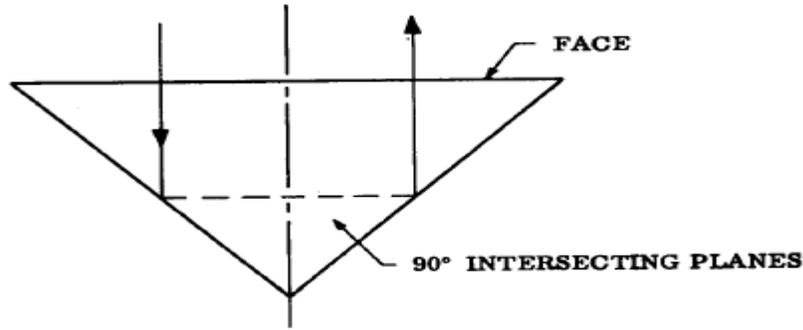
Figure 2.8 Reflection from a Trough from Huynen [2]
