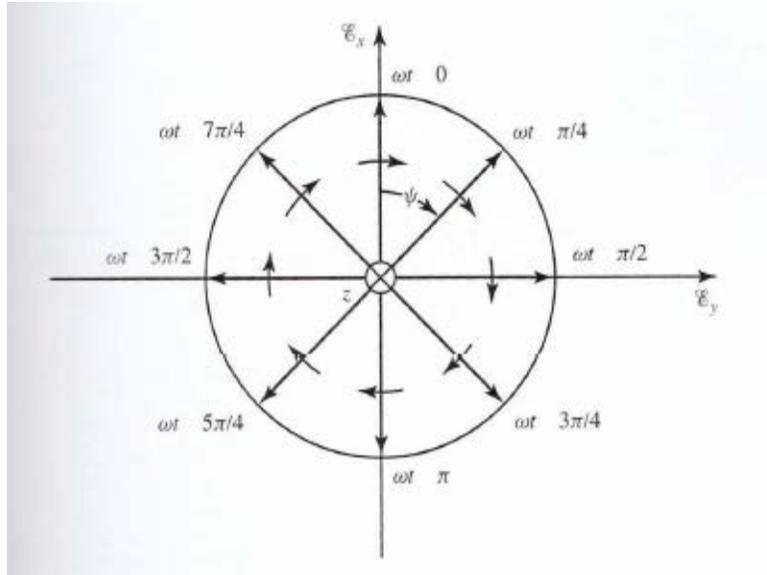
Figure 1.4 Right-Hand Circularly Polarized Wave from Balanis [9]
