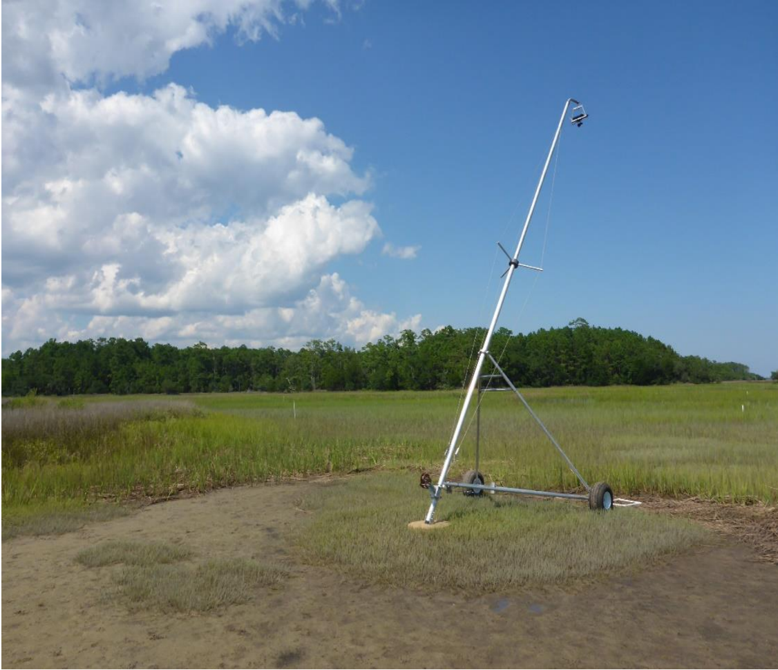
Figure 4.2: Depiction of the USC Prototype Machine Shop developed ‘howitzer’ used to hoist the Leica P20 in the saltmarsh.
