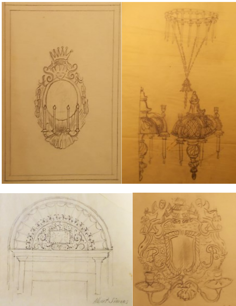
Figure 2.4: Sketches by Albert Simons of various architectural and decorative elements in the Dock Street Theatre. Beneath the bottom right drawing was the note: “One pair of William & Mary Silver Sconces, reproduced from those made by John Rand of London in 1703, Courtesy Crichton & Co.”
