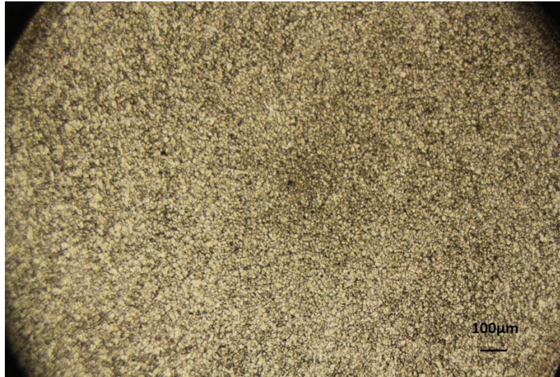
Figure 3.39 Fine equiaxed and recrystallized grain structure of AA6061 in friction extrusion wire, etched with Keller's solution for 180 seconds
