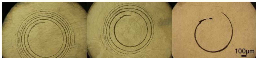
Figure 3.33 Spiral changes along the length of the wire extruded using the flat die with 400 rpm and 44500N, (left) 2.54cm from the beginning (middle) 7.62cm from the beginning (right) 12.7cm from the beginning
