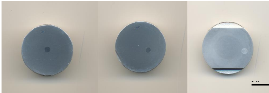
Figure 3.8. AA6061 Cylinder Samples with AA 2195 marker in center, 1/3 radius, 2/3 radius position respectively
