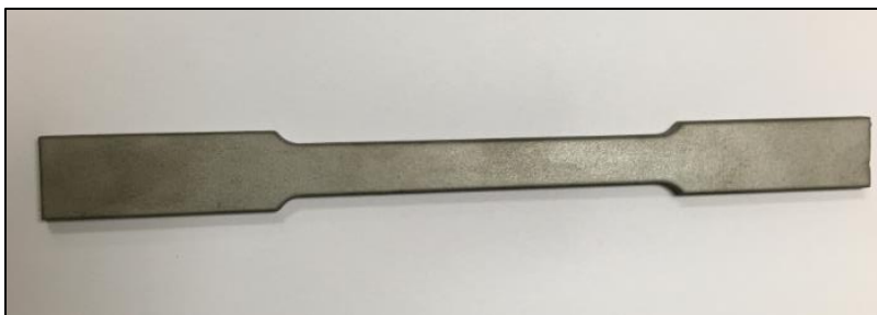
Figure 2.12. 304 Stainless steel flat dog-bone specimen cut using a CNC water jet
