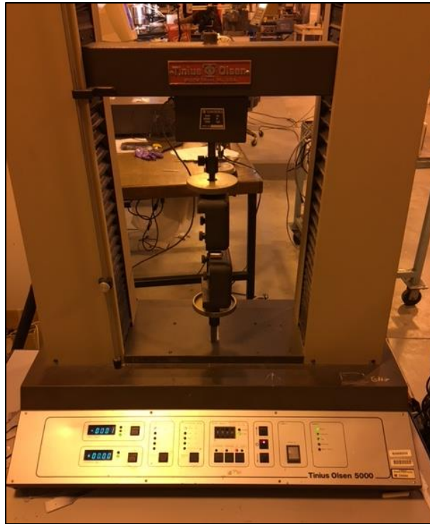
Figure 2.9. Tinius Olsen 5000 tensile testing machine
