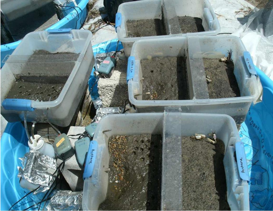
Figure 2.6 Crab feeding rate experiment photo. Mesocosm tanks containing field collected sediments were set-up and dosed with treatments. Four male fiddler crabs were introduced into one half of each mesocosm and allowed to feed for 24 hours. Measurements of sediment chlorophyll *a* concentration on each half of the tanks (crab exposed and crab excluded) were compared to determine the degree of feeding by the crabs.
