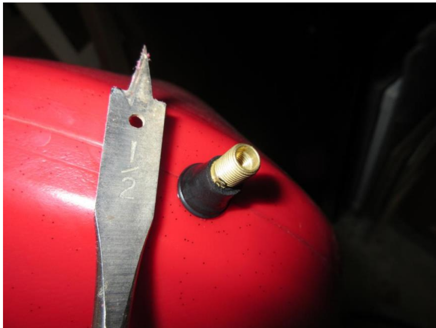
Figure 3: Gas can modified to allow venting
