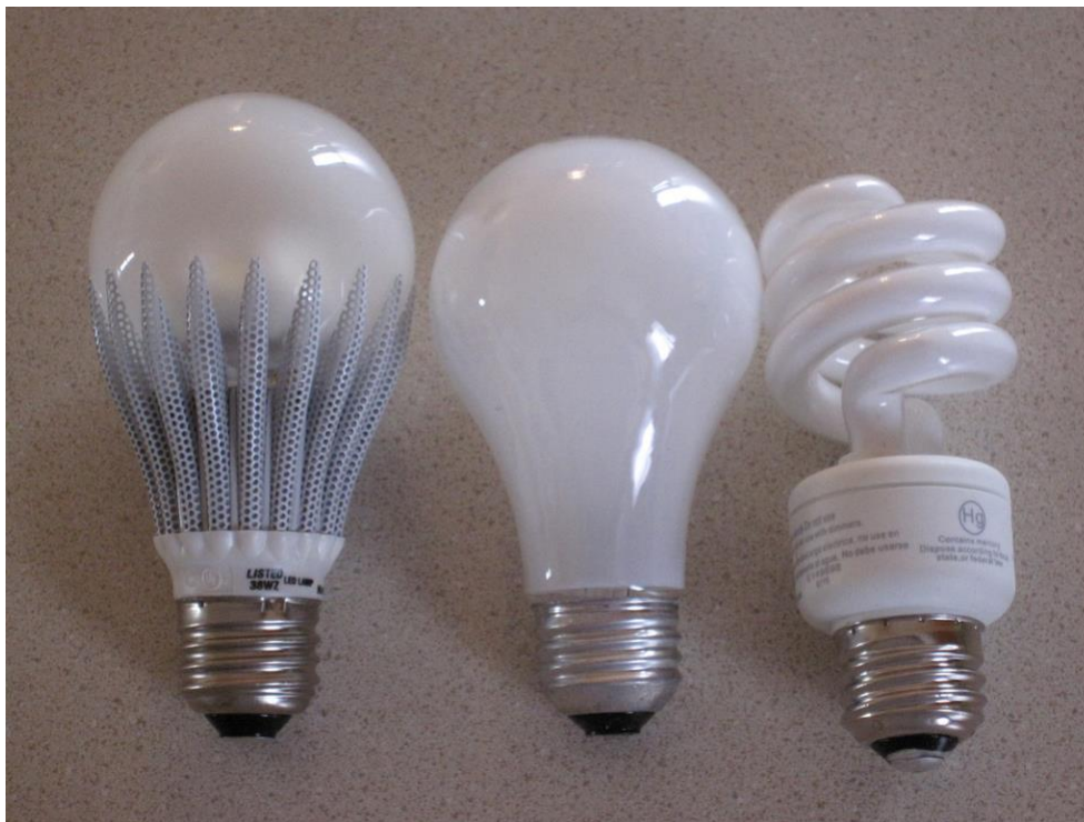
Figure 7: Light bulb technologies; from left to right, an LED, incandescent, and CFL bulb. All three produce roughly the same amount of light, but the incandescent bulb uses 60 watts of electricity to do so, while the CFL uses 13 watts and the LED only 7.5 watts. 80
