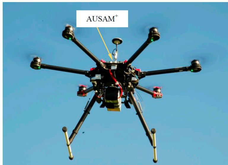
Figure 38. AUSAM + strapped on-board a SJ900 Hexacopter during flight testing.
