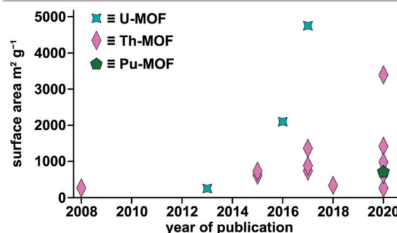
Fig. 5 (Top) X-ray crystal structures of Th_6(\mu_3-O)_4(\mu_3-OH)_4(BPDC)_4 , Th_6(\mu_3-O)_4(\mu_3-OH)_4(BPC)_4 , [Th_3(BPTC)_3O(H_2O)_{3.78}] \cdot Cl , and Th_6O_4(OH)_4(H_2O)_6(TBA)_6 . The pink, blue, gray, and red, spheres represent thorium, nitrogen, carbon, and oxygen atoms, respectively. (Bottom) Literature analysis of the surface areas of several reported An-MOFs over time. 3,59,66,78,134,138,159–163
