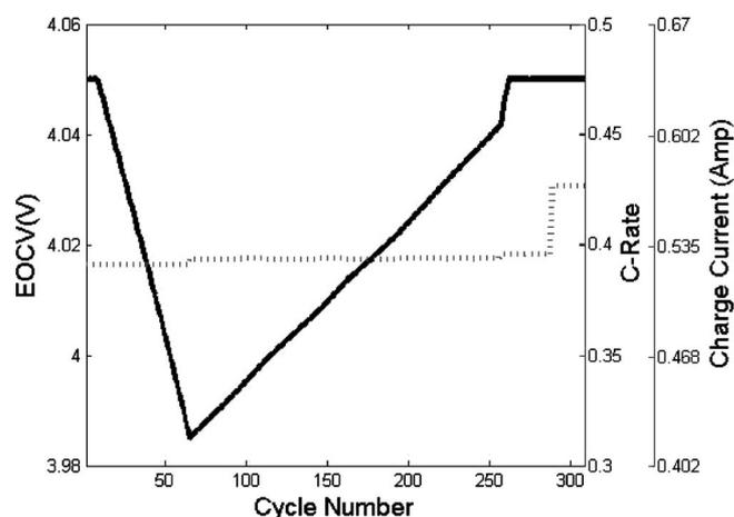
Figure 15. EOCV vs cycle number for 20 charge currents.
