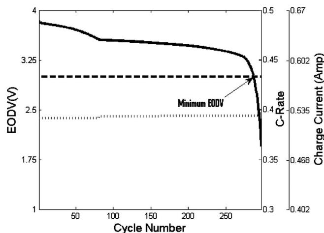
Figure 12. EODV vs cycle number for four charge currents [ $I_{app}(4) = I_{app}(3)$ ].
