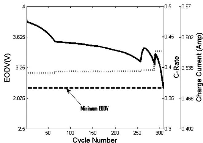
Figure 14. EODV vs cycle number for 20 charge currents.
