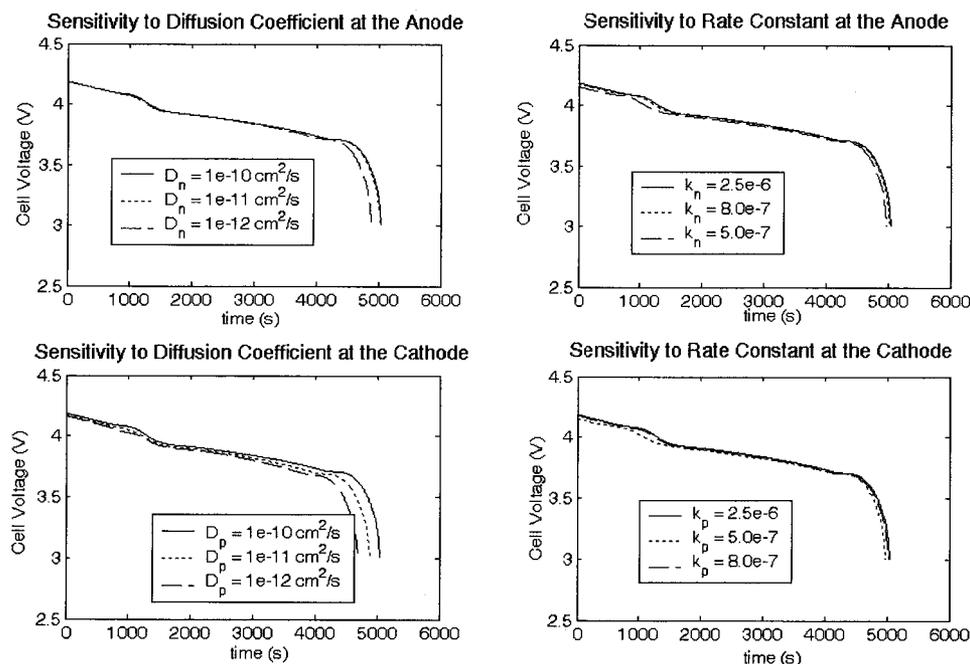
**Figure 3.** Sensitivity of the porous electrode model to the diffusion coefficient of lithium in the solid phase of each electrode and the electrochemical rate constants.
