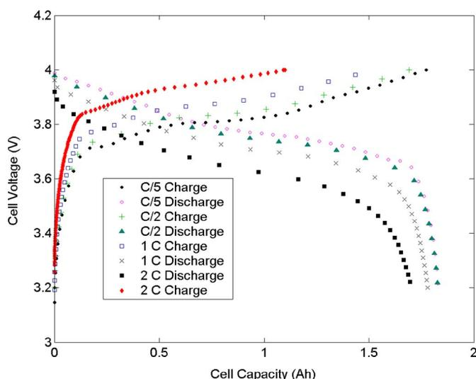
**Figure 2.** (Color online) A typical set of experimental data: four sets of charge and discharge curves corresponding to C/5, C/2, 1C, and 2C rates are shown.
