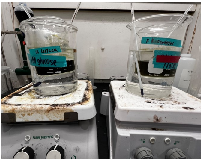
Figure 3. Evaporation Using a Water Bath. This figure displays the water bath setup used, in order to evaporate the remaining liquid in the extracts. Notably, the extract-filled beakers are positioned within a larger beaker filled with water, resting on top of hot plates. Additionally, each beaker is equipped with a thermometer immersed in the water, ensuring continuous monitoring of water temperature during the evaporation process.
