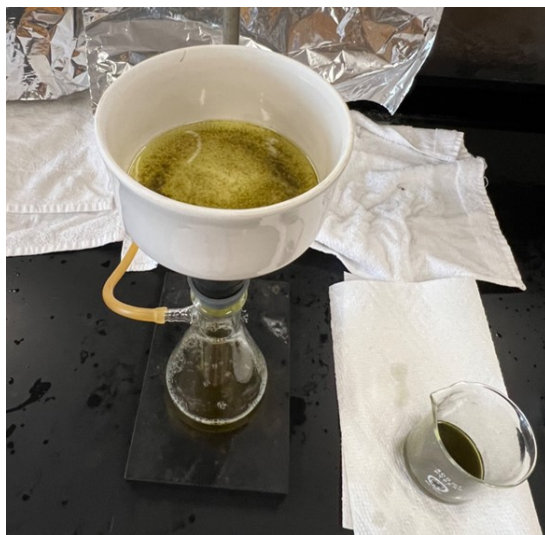
Figure 2. Vacuum Filtration of Algae Extracts. This figure displays the vacuum filtration setup, used for separating the extracts from the algae powder. Suspended by a ring stand, the setup features a side-arm flask on the bottom, with a Buchner funnel securely attached. Notably, the yellow tubing connects to a dual hose inlet adapter, establishing a vacuum effect by linking to a sink (not shown). Positioned in the bottom right corner is the beaker containing the algae extract
