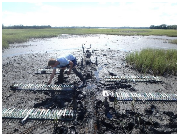
Figure 4. Photograph of undergraduate student (Jack Dekle) collecting biodegradable plastic strips from field-deployed apparatus in a salt marsh.
